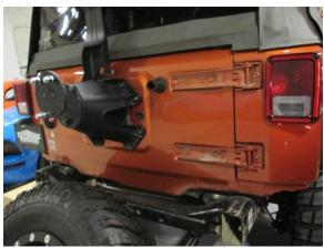
Step 1. Remove the rear wheel, then pull the hinge covers off by unsnapping them from the hinge assembly.
