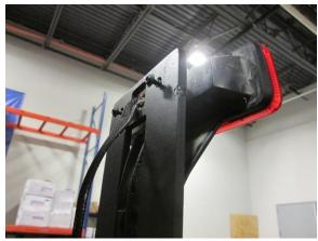
Step 10. Using the factory hardware, mount the brake light to the new bracket and route the wires into the door using the factory grommet and wiring harness.
