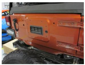
Step 2. Remove the (8) 10mm bolts holding the tire carrier to the rear of the vehicle.
