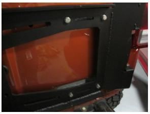
Step 6. Using the long 10mm bolts supplied with this mount, slide them through the carrier and through the supplied spacers to bolt it to the rear door. Note, the longer spacers will be used closer to the hinge for proper fitment.
