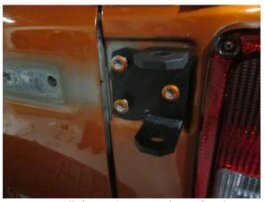
Step 4. Install the replacement hinge hardware to the factory mounting points using the factory hardware.
