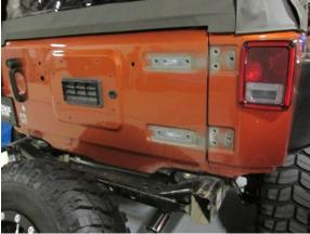
Step 3. Remove the (4) 10mm bolts holding the hinge to the rear door, then remove the (6) T-50 torx bolts holding the hinge to the body of the Jeep
