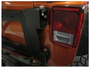
Step 5. Mount the new tire carrier to the hinges using the supplied 21mm mounting bolts and 22mm nuts to hold it in position.
