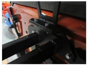
Step 9. Mount the third brake light bracket to the tire mount using the supplied 10mm bolts and nuts.
