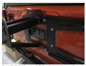
Step 7. Bolt the rest of the tire carrier to the rear door using the (8) 10mm supplied bolts. The mount will reuse all factory mounting points.
