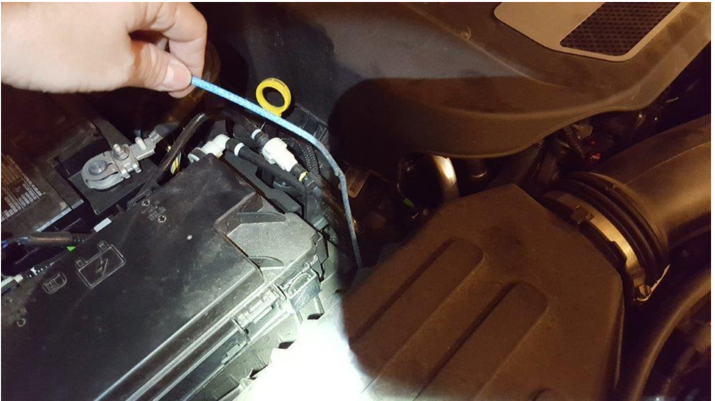
16. It's hard to see in the picture but here is where I routed the hanger between the wires and the frame. This will help hold the cables away from moving parts.
