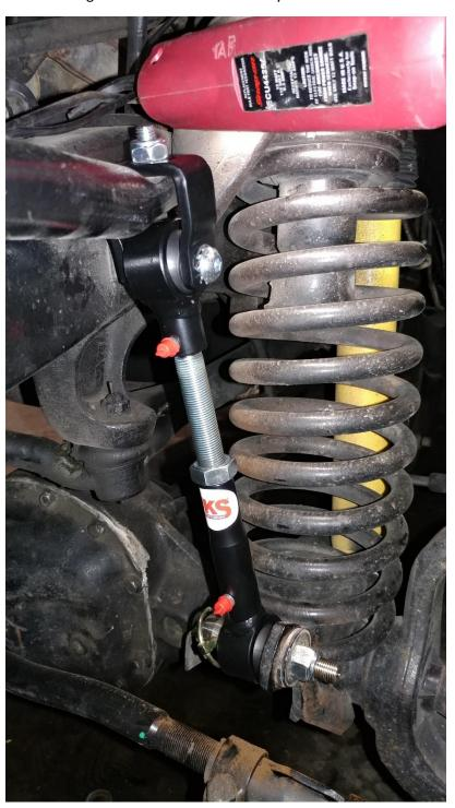
16. Slide the lower end of the sway bar link on to the post. Notice the amount of space, therefore I did not install the rubber spacer.
