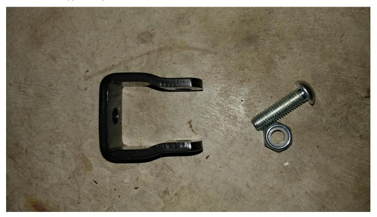
9. Using a 6mm Allen and 17mm socket tighten the provided hardware. The threaded side of the U-strap must face inboard
