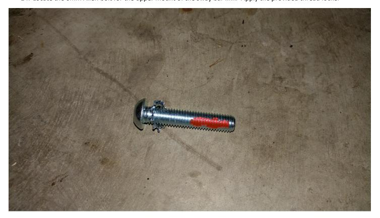
15. Using a 6mm Allen install the sway bar link
