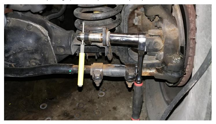
12. The post sat too far inside the hole not allowing the nut to fully tighten. I had to add washers to push the nut back to where the threads where.
