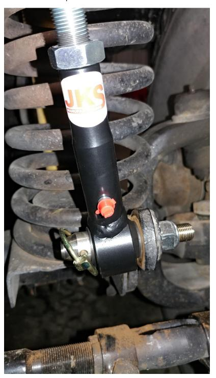
17. Set the angle of the sway bar per the 10-degree requirement. Using a crescent wrench tighten the locking nut.
