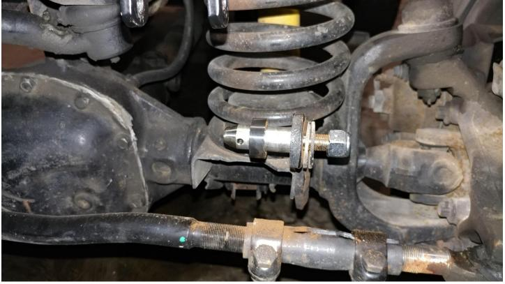
13. I also found that the provided rubber spacer did not allow for the sway bar link end and locking pin. So, I did not install the rubber spacer, seen in the final photos
