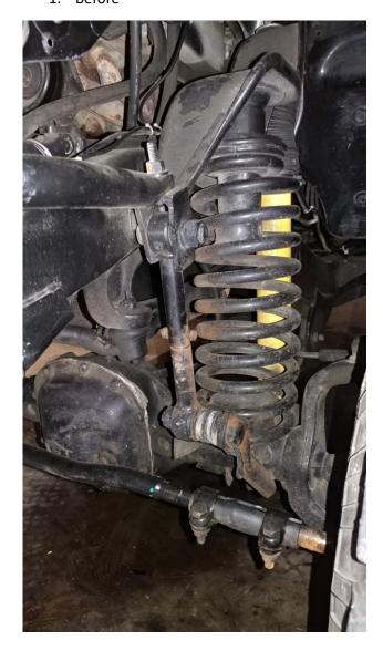
2. Using a 15/16 socket for the lower nut and a 1 - 1/16" socket for the lower bolt head remove the assembly
