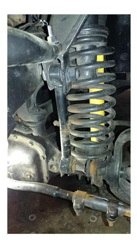
3. Using a 15mm socket for top nut. Remove it and this will release the existing sway bar link.
