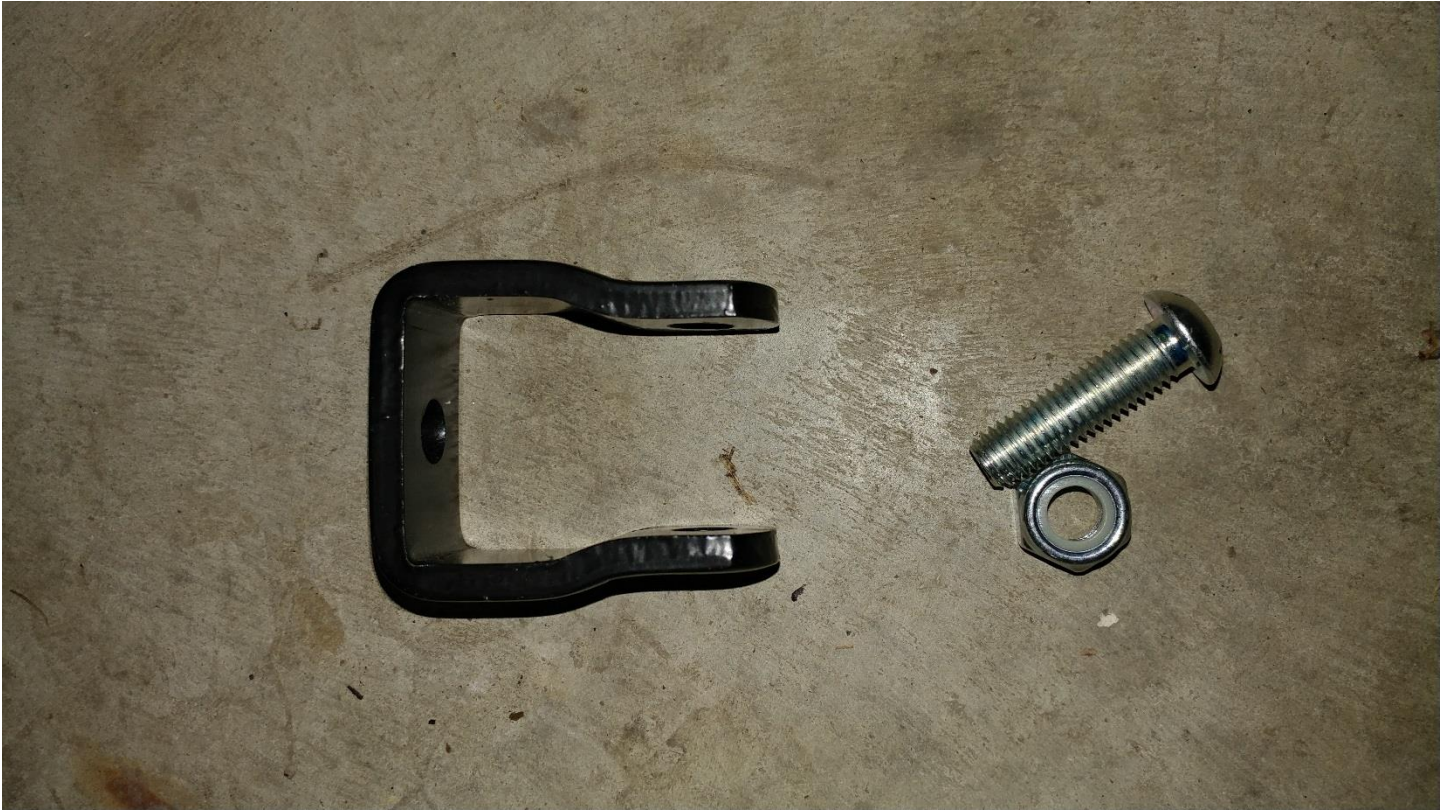
8. Locate the upper U-strap and hardware
