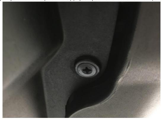
2. To remove clips, use a phillips head screwdriver to unscrew the center of the clip while not allowing the outer part to spin
