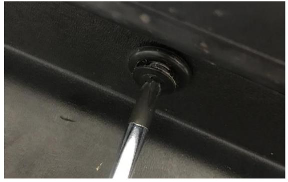
3. Once the center is unscrewed, the clip can be either pulled out or gently pried out with a flathead screwdriver or pry tool
