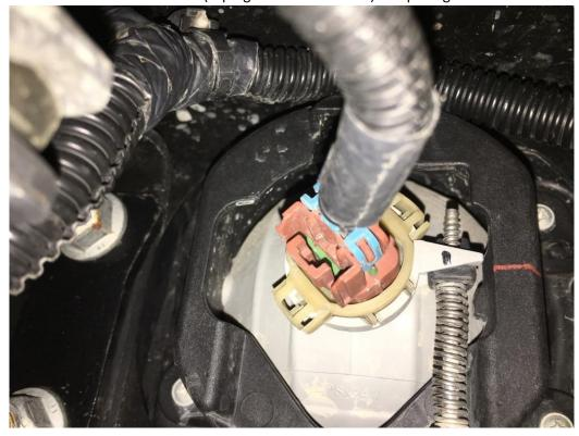
7. Remove the factory bulb from the red connector by simply pulling the bulb firmly from the connector
