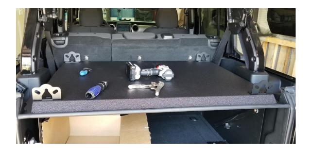
4. Once a gear anchor configuration has been decided upon, mark each hole carefully with a marker or pencil and drill pilot holes with your 3/8<sup>th</sup> drill bit.
