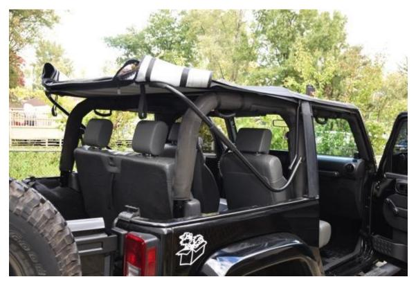
3. With Phillips head screwdriver remove four screws on rear bow and place to side for later.
