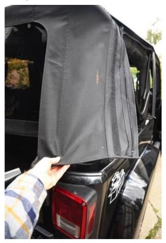
16. Go inside Jeep and look for four tabs in top by back bow and screw tabs to back bow with the four screws you saved from earlier.
