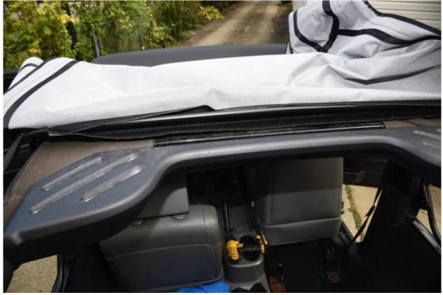
5. Unhook sides of top from belt rails on passenger and driver side. Unlatch both clamps that hold main header down.
