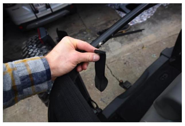
15. Pull back top more to back bow and pull ends down towards ground. Give a good tug on both sides for snug fit. Then place backside belt rails to back channels.
