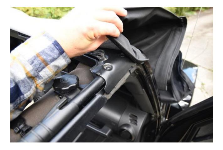
12. Flip top back off windshield and drape towards back of Jeep. Lift main header up and replace four screws underneath both left and right side. Now all screws will be in main header and you can clamp back down main header to
