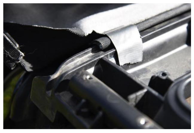
11. Place about four pieces of duct tape evenly across main header channel so the top doesn't move on you. Then replace plate on main header, screw in left and right top screws and tuck the sides of new top over main header, there will be pocket like stiches on both sides. Replace all screws to plate on main header.
