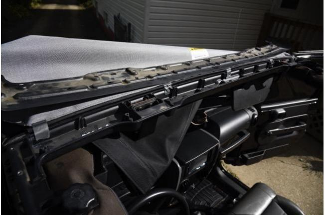
10. Take new top and look for front. New top will have a small plastic tube like piece stitched in at front. Pay close attention so that you have the correct side facing down. Place this neatly in channel of main header.
