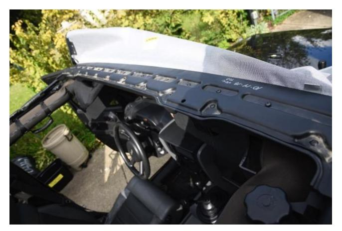
9. Once all screws from main header are removed, take off plate cover on main header (take a good look at how the old top is placed in for easy new install) and remove the old top.
