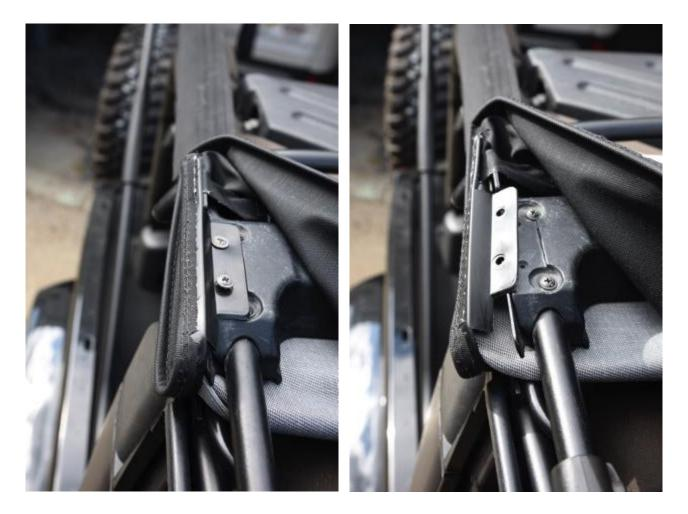
7. Flip main header back to front of Jeep and CAREFULLY place cover over windshield.
