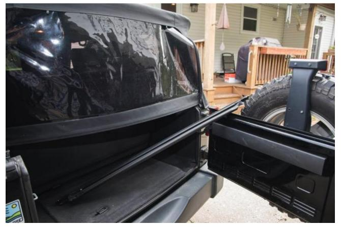
18. Zip up side windows left and right and place belt rails to side channels.
