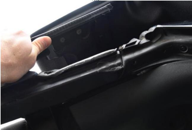
13. Pull top back and Velcro center of top to center bow. And then put driver and passenger side belt rails into side channels.
