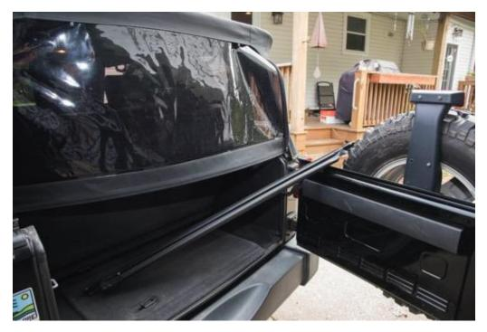
2. Pull down rear corners and remove from belt rail. Do this for both sides and flip up onto roof.
