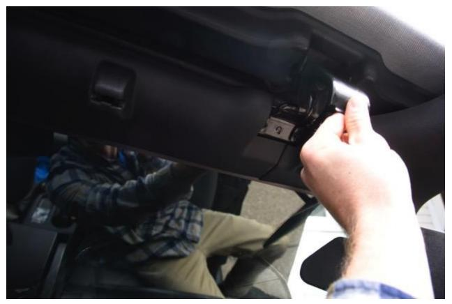
6. Underneath main header (left and right side) there are two screws followed by two more. Helps to flip main header back for easy access. Remove all four screws on header left and right side (Save for later)
