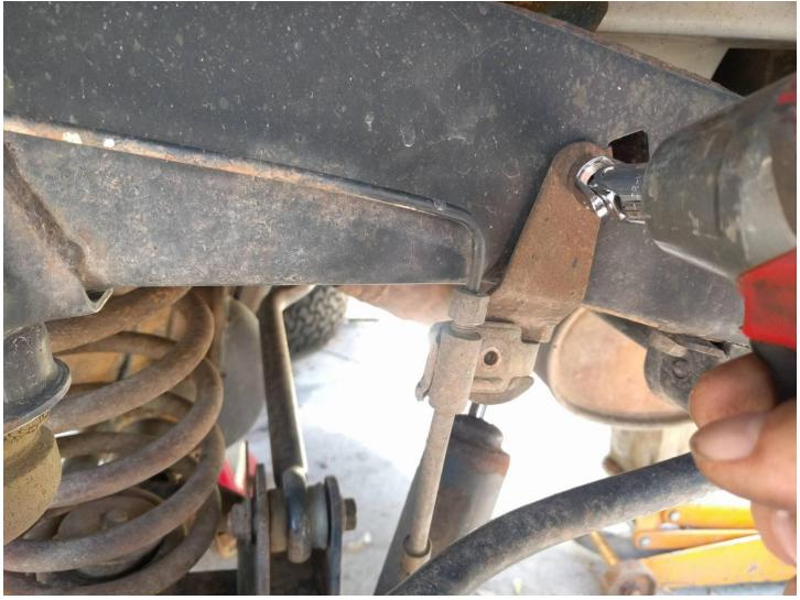
4. Taking care to hold vehicle-side hardline steady and not kink or fracture line, slightly loosen compression fitting with flare or box wrench and then rotate old rubber brake line to remove. Again, it's very likely that the compression nut on your hardline will not rotate without twisting and eventually breaking the hardline, so rotating the extension line while holding the compression nut steady is recommended. That's why you removed the caliper end first.
