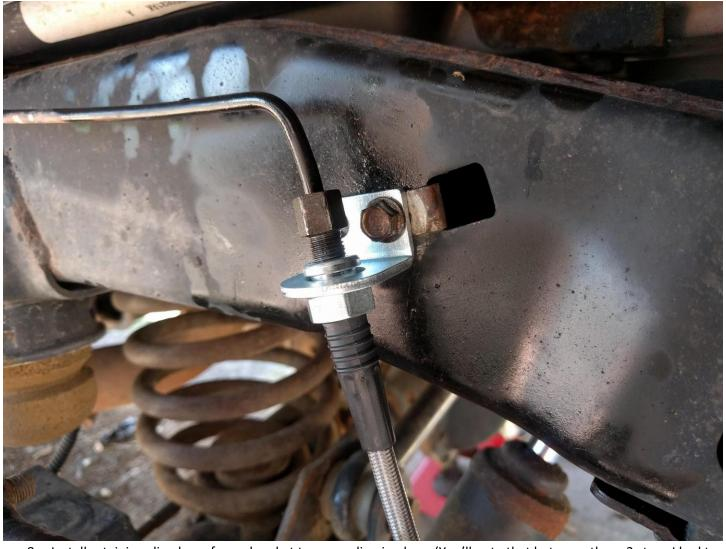
8. Install retaining clip above frame bracket to secure line in place. (You'll note that between these 2 steps I had to go back and flip the bracket due to too much stress on the hardline as I tightened the fittings. Though Teraflex directions showed the bracket the way I initially installed it, you can see in the photo below that with it flipped the hardline sits along top edge of frame where intended.)
