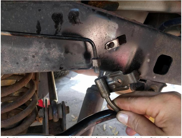
5. Using new copper crush washers provided, and reusing factory banjo bolt, secure banjo eye fitting to caliper. Several thicknesses of copper washers are provided with kit, use appropriate combination to center bolt drain hole in banjo fitting.
