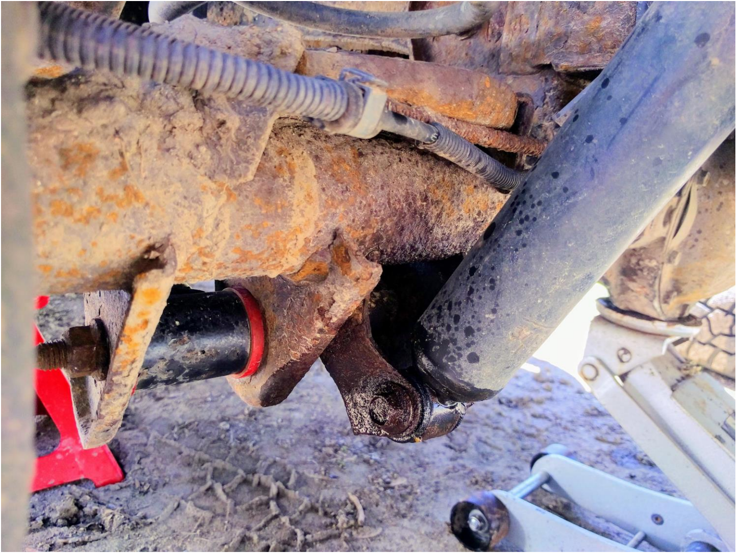
8. Reconnect Sway Bar End Links - Torque spec is 40 ft-lbs.
