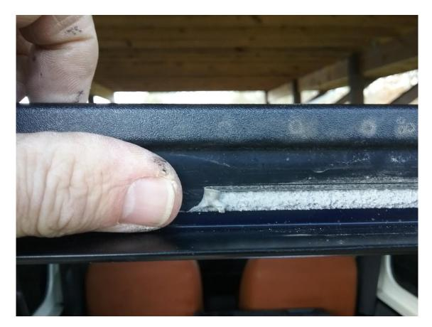
After removing all the old adhesive, use an alcohol wipe or a rag dampened with rubbing alcohol to thoroughly clean the mounting surface. Prior to installing the new seal, the mounting surface should be clean and completely free of any adhesive or foreign material to ensure proper adhesion of the new seal.
