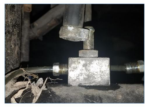
12. Use 9/16 wrench to remove axle breather tube from the junction box and remove the brake hose. Retain the breather tube and bolt.
