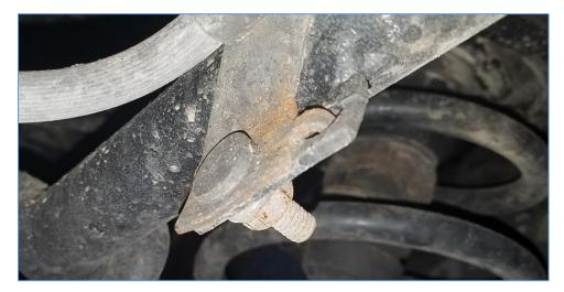
10. Use T40 Torx wrench to remove Torx bolt securing the brake hose on the frame side. Allow the line to drain into the catch pan. Use Torx bolt to secure the new bracket to the frame and attach the new brake hose to the brake line. **TIP:** Doing this now will stop brake fluid from dripping down while removing the axle junction box.
