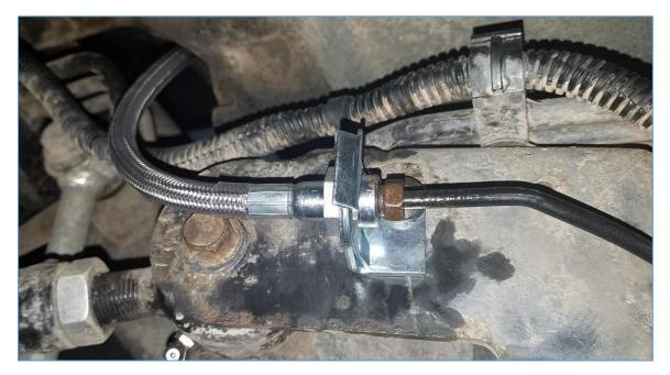
**TIP:** Tuck the new brake hose up out of the way to prevent the brake fluid from draining down.
