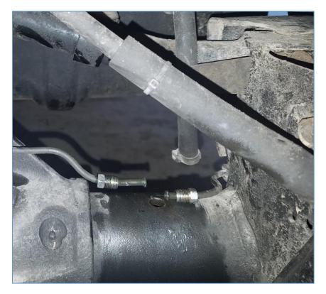
13. Re-install breather tube bolt through the new brake hose and attach brake lines to the junction box. **TIP:** Since hard brake lines may not line up with the new box, start a couple threads on each brake line before securing the junction box to the axle with the breather tube bolt. Once all lines are connected, tighten the flare nuts and breather tube bolt. Re-attached breather tube to the axle.
