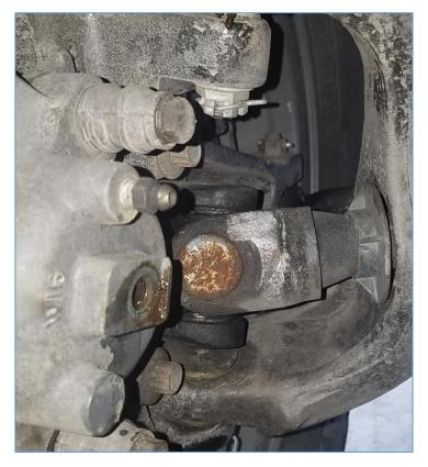
4. Use Torx bolt to secure new hose bracket to the frame. **TIP:** Use a little anti seize compound on the bolt.
