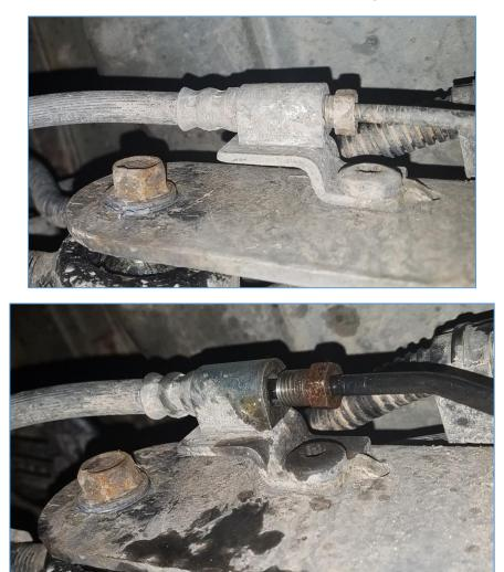
9. Use 13 mm wrench to remove nut holding brake hose to the rear Driver side upper control arm.
