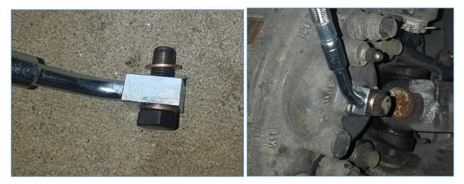
6. Place new hose coupling (frame side) through the hole in the bracket and secure with the clip. Use a mallet or hammer to secure the hose clip. Attach brake line flare nut to the new hose. Use 18 MM box wrench to hold the nut on the new brake hose while tightening the hard brake line.
