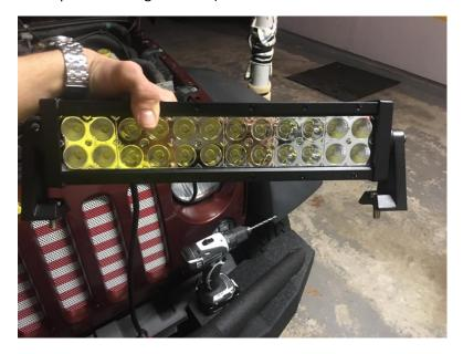
3. Place the light bar on the bumper and mark where the bolt holes must be screwed. Then screw into the bumper with a 5/16 drill bit so that the light bar can be bolted to the bumper.
