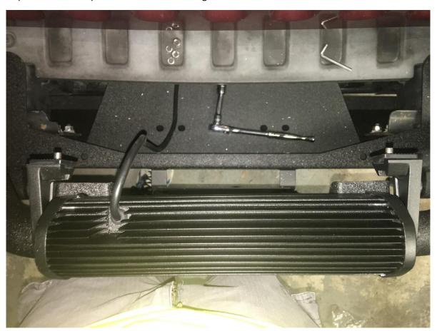
5. Place the light bar on the bumper, making sure the bolts go into the holes that you have just screwed.
