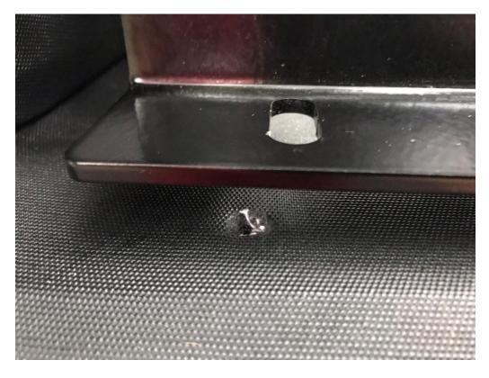
4. Secure the "L" bracket to the body of the car (do not tighten all the way) with OEM bolts on both sides.
