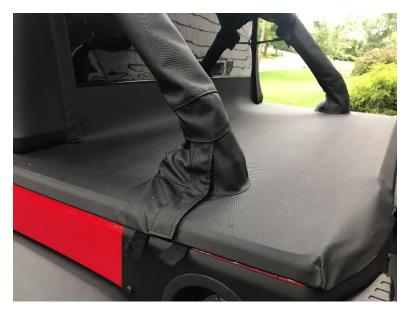
2. Position the rack between the roll cage by loosening and removing aluminum inserts on both sides and replacing once positioned around roll cage.
