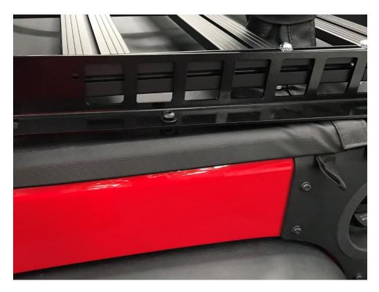
5. Place covers over the "L" bracket and align bolt openings with supplied nuts (to be inserted in open channel of rack)
