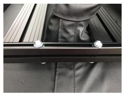
3. Position the "L" brackets along each side of the cargo rack, aligning "L" bracket with existing jeep inserts in the body of the jeep. If necessary, make holes in the cargo top large enough to use OEM bolts.
