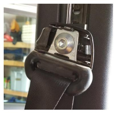
6. Remove B-pillar trim by pulling it towards the inside of the Jeep. If plastic clips remain in the B-pillar, remove them and re-install in the trim piece.
