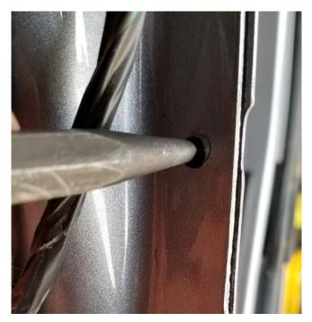
11. Drill using 1/8 inch bit first, then finish with 1/4 inch bit.
