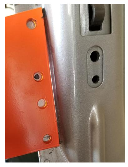
10. Remove harness bar and center punch holes.
