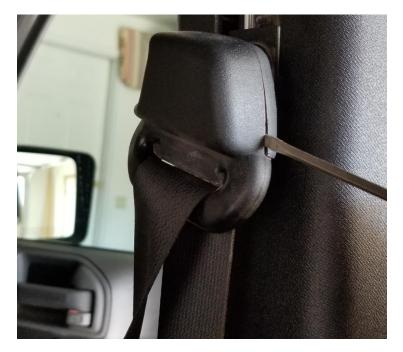
5. Using T50 Torx, Remove upper seat belt bolts from both front seat belts
