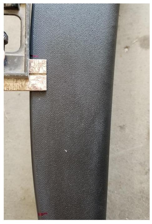
19. Using a combination square, draw a line 1/2 inch in from the top tine to the bottom line. Since the trim piece is curved, it's hard to get a curved line without using this type of square. Put a marker at the end of the ruler, and move the ruler down the trim piece. It will create a near perfect curved line to cut on.
