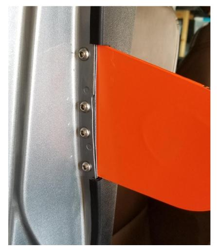
22. Reinstall seat belts, torque T50 Torx bolts to 29.5 ft lbs.
