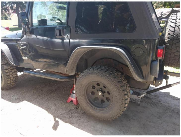
2. Locate and remove both sway bar end links (18mm bolts).
