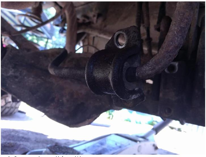
4. Remove sway bar assembly from vehicle.
