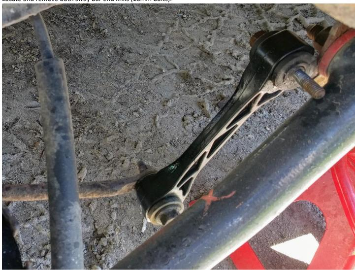
3. Locate and remove all 4 sway bar mounting bolts (15mm Bolts).
