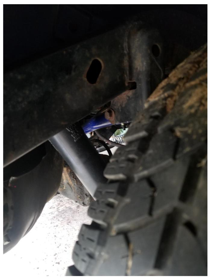
Lower jeep down and can now adjust the track bar to center axle under jeep using crescent wrench and tightening the lock nuts down pictured in step 6.
