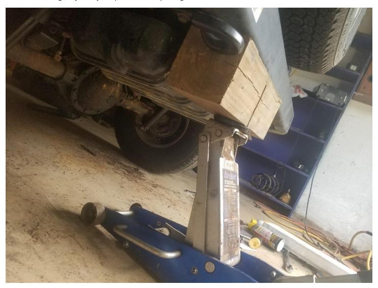
2. Now using the jack to jack up the rear bumper to gain access to the T55 torx bolt on the axle side bracket.
