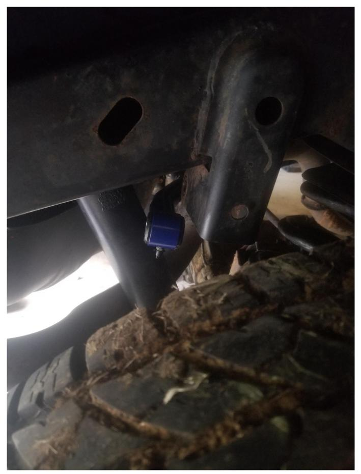
6. Install into bottom bracket grease fitting facing down and use the tab nut and T55 torx bolt and torque to 74 ft-lbs. all year models.
