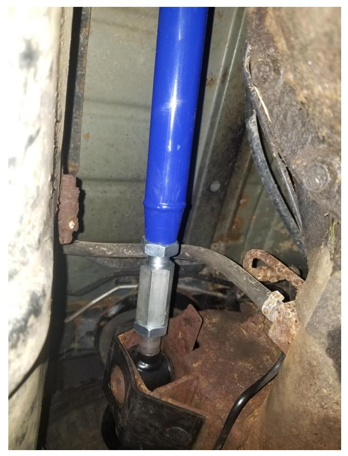
7. The track bar will not go into the frame side bracket because the stock exhaust is in the way. I cut the exhaust behind the muffler temporally until I can go to exhaust shop to run some custom exhaust.
