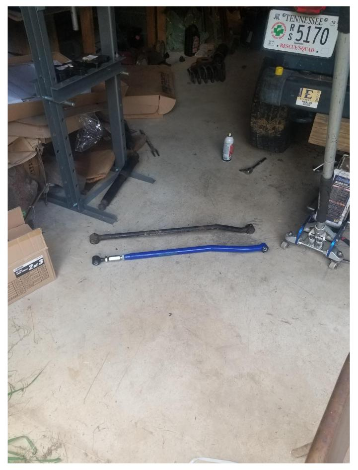
5. Install new track bar with the adjustment end towards the bottom making sure the top part goes over exhaust with the company logo facing out the back.
