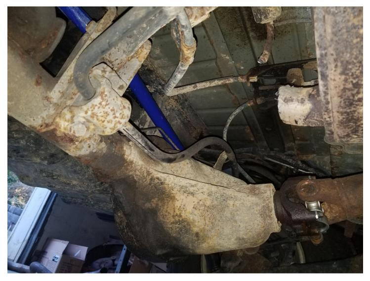
8. Once the exhaust is out of the way, the top of the track bar will go into the bracket and the bolt goes in from back side of the bracket. Torque this bolt to 74 ft-lbs. for all Jeep Wrangler years.
