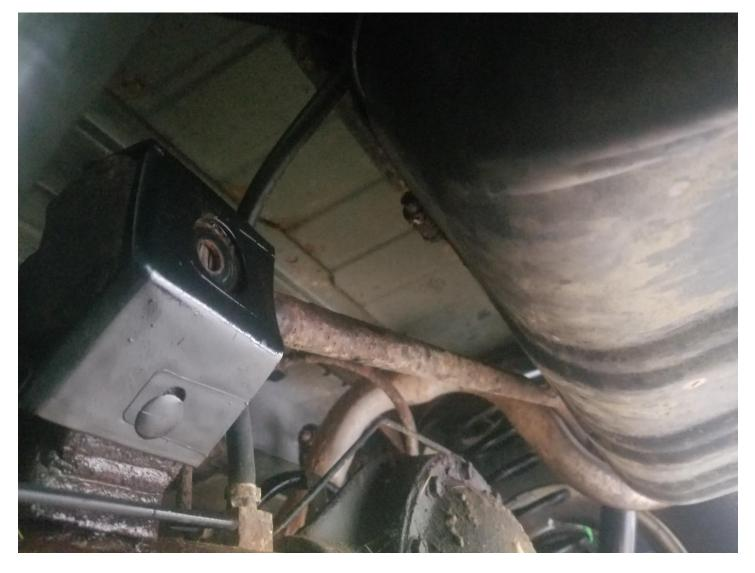
4. Remove old track bar by pushing it out of the lower bracket; then side it out towards the driver side.
