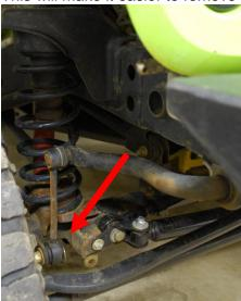
3. Use a 21mm wrench to remove the two (2) track bar bolts (one on each end) and nuts. Remove old track bar and set aside.
