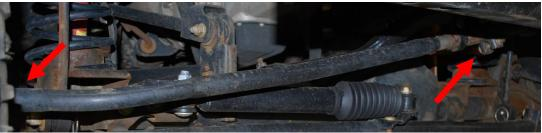
4. Align new track bar by adjusting the turn-buckle until the track bar bushings and bracket holes line up, and insert two (2) 21mm bolts through track bar bracket and track bar. Tighten bolts/nuts to 125 ft-lbs.
