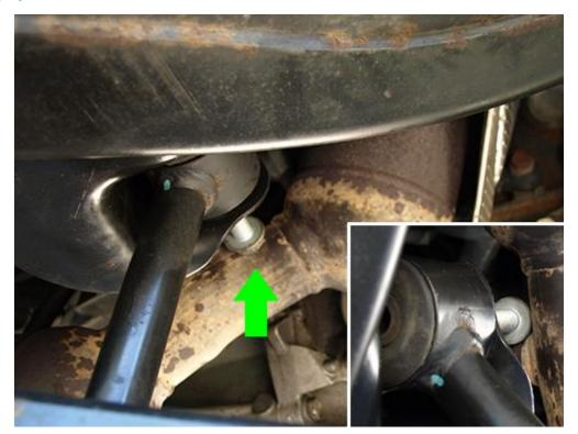
6. Place the factory 18mm bolt through the axle front mount and upper Steinjager upper control arm. Loosely place the nut on the bolt. Do not tighten. Important Note: You may need to move the axle around a bit to get the holes to align. Be extremely careful when doing this.
