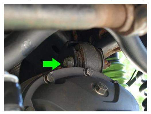
4. Break free the 18mm rear upper control arm bolt using an open ended 18mm wrench. (A ratcheting wrench is recommended. Depending on your make and model. The rear bolt may be very close to the exhaust and a socket wrench will not fit.) There is a flag nut on the opposite end.
