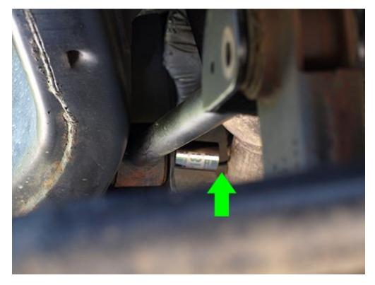
5. Slowly twist the factory passenger side upper control arm if the factory bolt comes into contact with the exhaust when trying to remove it.
