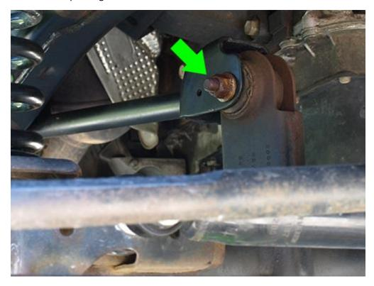
The driver side upper control arm is bolted to the mount that is right above the pumpkin.
