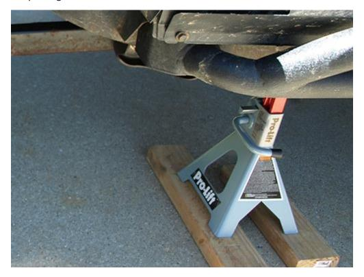
2. Support the front axle with jacks stands and remove the front tires.
