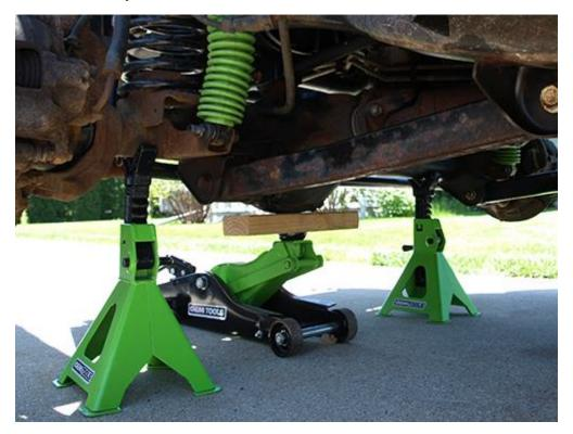
3. Using a 18mm open ended wrench and a socket wrench with a 18mm socket. Break free the front upper control arm bolt and nut on the passenger and driver side. Remove the 18mm bolt from the hole.
