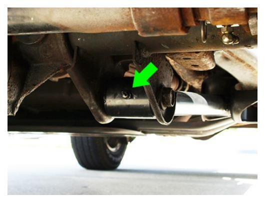
Note that the rear Zerk fitting will be the most challenging to grease because of how close the fitting is to the frame.
