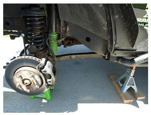
3. Using a 21mm open ended wrench and a socket wrench with a 21mm socket. Loosen the front lower control arm bolt and nut on the passenger side. Leave the bolt in to prevent the control arm from swinging down while breaking free the rear bolt.
