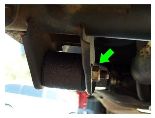
4. Using the same 21mm open ended wrench and a socket wrench with a 21mm socket. Loosen the rear lower control arm bolt and nut. Now remove the front and rear bolts and slide the factory control are out.
