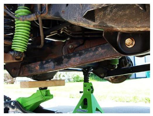
7. Place the tires back on the Jeep<sup>®</sup> and remove jack stands. With the Jeep<sup>®</sup> on its own weight. Torque the lug nuts to 95-foot pounds and the lower control arm bolts to 125-foot pounds. You will need to grease the Zerk fittings on front and rear of each lower control arm. Remove the Zerk cap off and grease the lower control arms using a grease gun.
