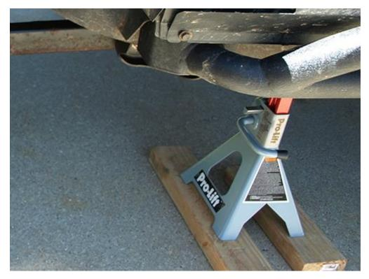
2. Jack up the front axle and remove the front tires. Support the front axle with jack stands.
