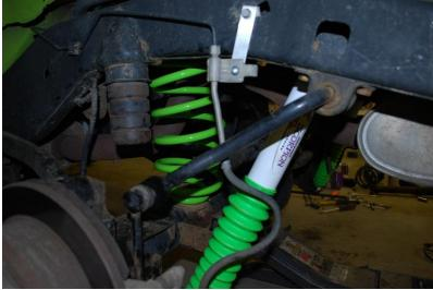
16. Reinstall the rear track bar using a 21mm Socket and ratchet, but do not fully tighten the bolt at this time.
