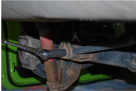
6. Using the 21mm Socket and Breaker bar, loosen the lower and upper control arm bolts. Do not remove the nuts completely, you just want these loose enough to make the differential swing down easily.
