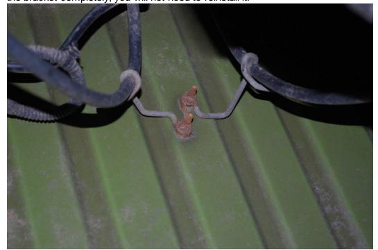
8. Using a 10mm Deep Socket and ratchet, remove the bolts holding the rear brake lines to the frame above the axle. In the picture, you will see brake line extension brackets installed. These do not come with the springs, but it is recommended to either make or purchase a set to ensure your brake lines will not bind.
