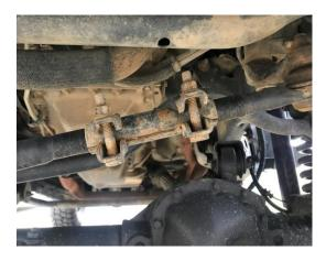
5. Take your new top mount drag link and screw it into the adjusting sleeve. Screw it in the exact number of times as you did when you unscrewed it. If you're installing a top mount draglink using the
