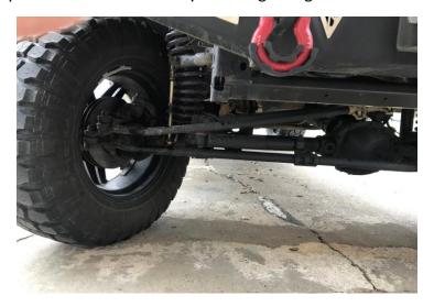
2. Loosen, without removing the ball stud nuts on the tie rod assembly using a 21mm socket.
