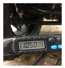
7. Make sure toe and clear vision (straightness of steering wheel) are set correctly and all nuts are tightened to the specified torque. The last step is to grease both drag link sockets through the zerks until grease purges around the boot seal; wipe off excess grease.
