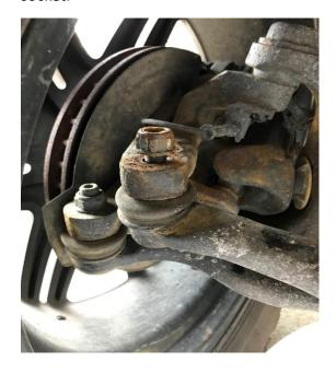
3. Unscrew the nuts until the top of the nut is above the end of the ball stud to prevent damage to the ball stud. Using a hammer, break the stud tapers loose separating the studs from the knuckles, and remove the drag link from the knuckle
