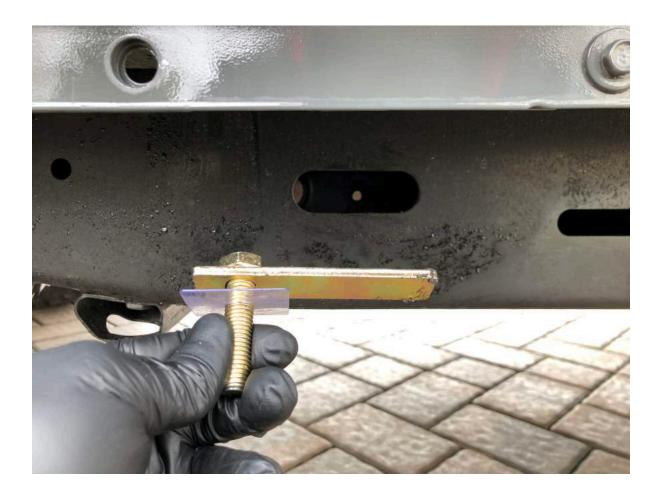
4. Slip the M10 U-Bolt through the bottom of the frame and rotate it through the second hole. Once the U-Bolt is in place, attach the two M10 Poly Retainers to keep the U-Bolt in place.
