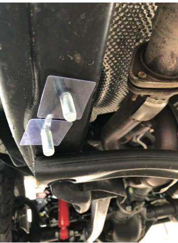
5. Now using your jack or an extra set of hands lift the rock rail into place and align the mounting locations. Start by positioning the rear and center body mount bolts. Once those locations are in place move to the front of the vehicle and line up the Bolt Plate and U-Bolt.
