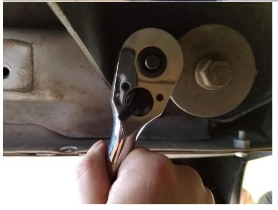
3. Align the snyper rail with your Jeep. The four bolts will slide through the openings of the rail. Have a second person hold the rail so you can begin to tighten the nuts. Tighten all four factory nuts with the four washers that were supplied. Do this by hand to begin with. Then tighten all four nuts using a torque wrench. You will need a deep socket 16 mm or a 16 mm with an extension. With a torque wrench, tighten all four nuts to 30-35 ft per lb.
