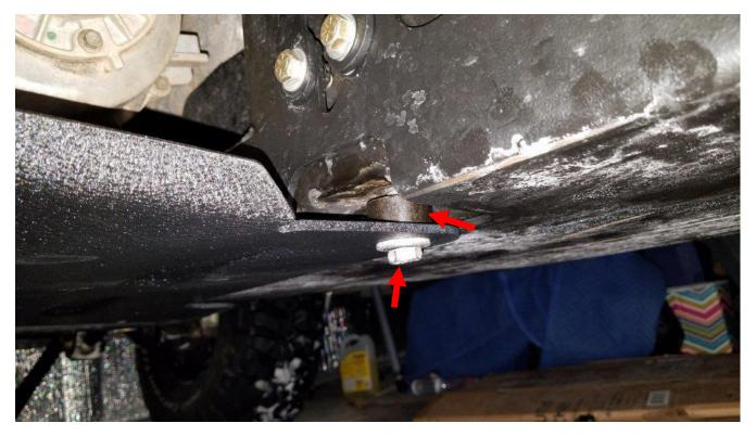
7. Next, tighten all the bolts. I recommend hand tightening them all, then fully tightening them using an 18mm socket. Torque them all to 48ft/lbs, including the 2 skid bar bolts loosened in step 3. Note: I was unable to get the middle bolt hole to align on the crossmember, probably because my crossmember is bent. If you have trouble with it, the skid plate is ok with only the other 4 bolts.
