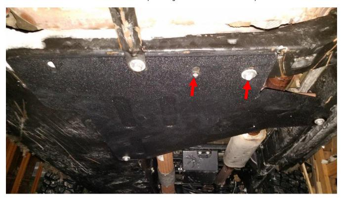
**6.** Now use the stock bolt with the supplied bolt spacer to attach the skid plate to the gas tank.
