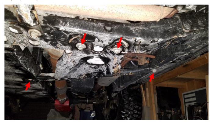
**3.** Using an 18mm socket, loosen the 3 bolts holding the stock transmission skid bar. *Note: If you are still using this stock skid bar then just loosen the bolts, but if you are getting rid of it you can remove it now.*
