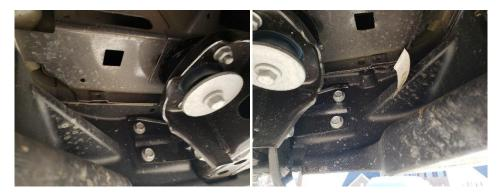
7. Now the factory bumper is loose and can be pulled back and removed.
