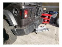
8. With a 21mm socket, remove the bolts holding the bumper bracket to the frame.
