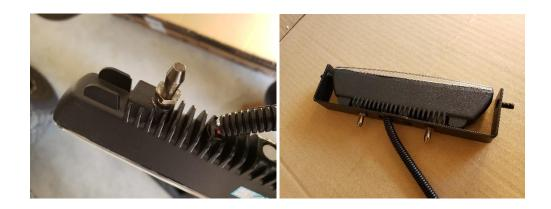
14. Install the light brackets to the new bumper.
