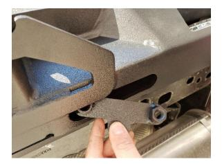
17. Secure the rear bumper to the rear frame crossmember using the four supplied 12m x 100mm bolts, washers and nut plates installed in the previous step.
