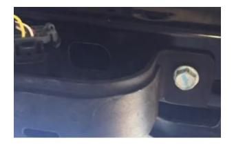
b. the four 18 MM bolts holding the receiver hitch to the frame cross member.
