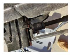
9. If equipped, remove the four 21 MM bolts holding the factory tow hook to the frame.
