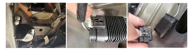
5. Using the trim removal tool, detach the three Christmas tree type pins holding the wiring harness to the frame.
