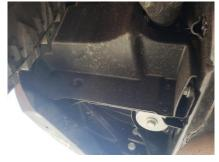
2. Using a 16 MM socket, remove the side rear corner brackets. There are a total of four bolts holding each of the two brackets (passenger's side shown).
