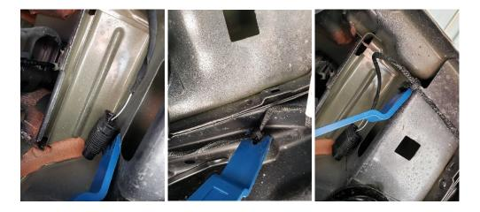
6. Now remove the four 16 MM bolts holding the factory bumper. Both passenger and driver sides are shown below.
