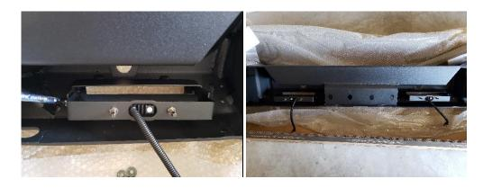
15. With the help of someone else, raise the bumper against the frame rails and align the mounting holes. Loosely secure to the outer frame rails using the previously removed factory screws.
