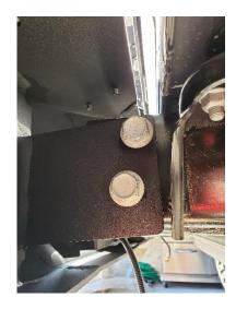
Different from the factory bumper, you will not be able to rest the new bumper on the frame while attaching with the hardware. You will have to hold it in place until, at least, one bolt have been placed on each side.
