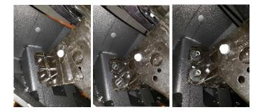
15. With the bumper center-aligned, you can now tight all eight 12 mm nuts to 70 ft-lb. Also tight the two 16mm bolts securing the lower portion of the bumper to the frame and the four 16mm bots holding the factory bracket.
