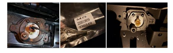
c. For JLs with the led package and the led light housing shown below, install the fog light adapter (84-401RM010) in the mounting stud and secure using the provided hardware (part no. Z30349).
