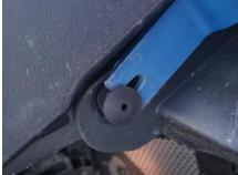
2. Using a trim removal tool, remove the two clips in the top of the bumper.
