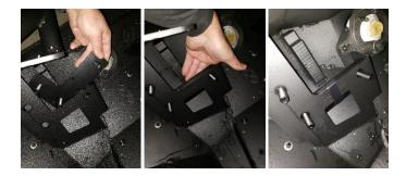
11. With the help of a friend, lift the bumper up in place and align the 3 mounting studs in each side with the holes in the frame mounting plates. Secure the bumper using the eight 12mm nuts supplied but leave them loose. This will ease installing the lower mounting tabs in a later step.
