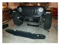
7. Using a 16 MM socket, loose the bolt holding the bracket attached to the frame. You don't have to remove the bolt. Just let it loose so you can leave the bracket temporarily hanging. This will ease installation of the bumper in a later step.
