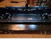
b. Using the trim removal tool, detach the clips securing the factory wiring harness to the factory bumper.
