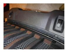
3. Using a 16 MM socket, remove the two bolts securing the metal skid plate. Then slide the plate up and detach.
