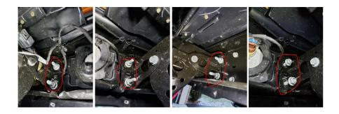
6. Ensure that nobody is behind the work area and completely remove the two nuts left for safety. Now the bumper is loose and can be carefully removed.
