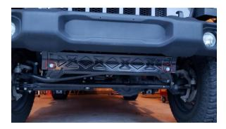
4. Detach the wire harness in the passenger's side. Press the locking tab and then pull.
