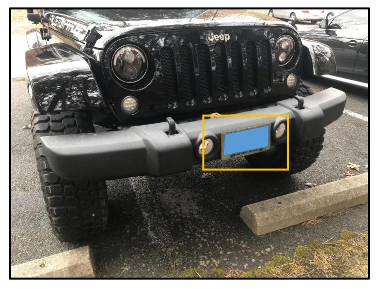
2. Remove the OE plastic frame cover, which sits behind the stock bumper and is held in place with two plastic fasteners. A screwdriver will allow for removal of the fasteners. It is then possible to slide the cover to the left and right to allow access to bumper attachment nuts.
