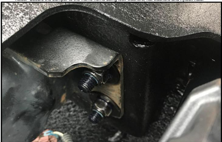
11. To fully secure the bumper to the frame horns, insert the 12 x 40 mm hex bolts along with lock washers and flat washers through the newly-drilled holes (which were enlarged in step 4) and tighten. Torque all bolts and nuts which attach the bumper to the frame horns to 60 ft-lbs.
