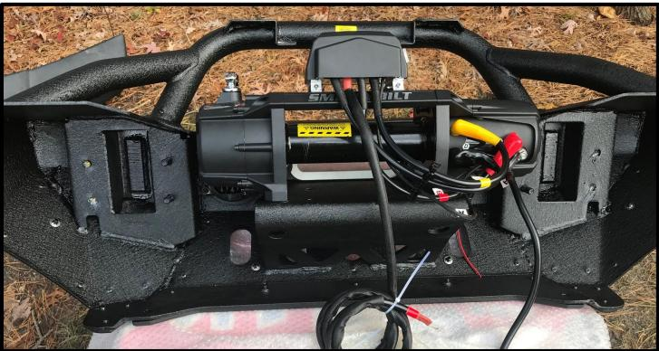
9. Locate the two bolts on each side of the bumper which will be used to attach the bumper to the frame horns of the Jeep.
