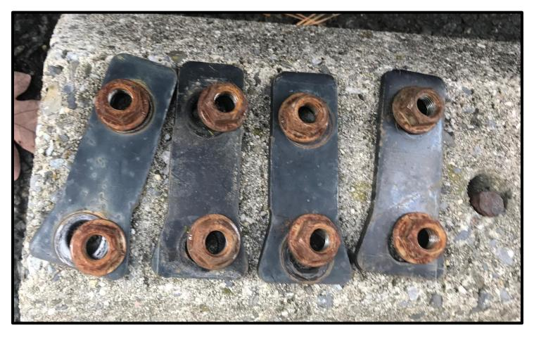
4. The outer frame horn holes will need to be opened up sufficiently to allow insertion of the bolts through the horn into the bumper. Smittybilt installation instructions call for opening the outer holes to 1/2", but a larger (or lower) hole may be needed to allow for full access. Failure to make the hole large (or low) enough will result in the second photo- (the bumper had to be removed again after install to enlarge and reposition the hole in the frame horn).
