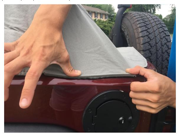
6. Slip the final two plastic pieces under the body near the tail light.
