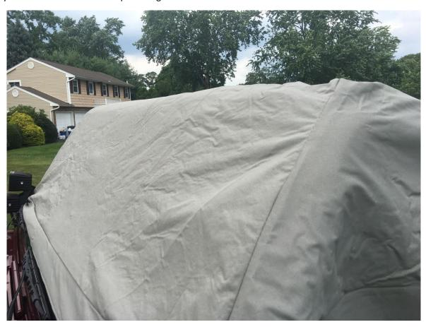
4. Slip the plastic piece of the cab cover underneath the body of the Jeep near the rear.
