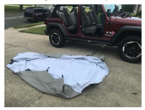
3. Lay the cab cover over the Jeep and align the corners of the cab cover to the corners of the windshield.
