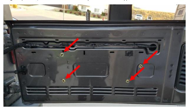
**14.** Using a 3/8"-16 nutsert tool, install all 4 nutserts. Then check to make sure none are loose.
