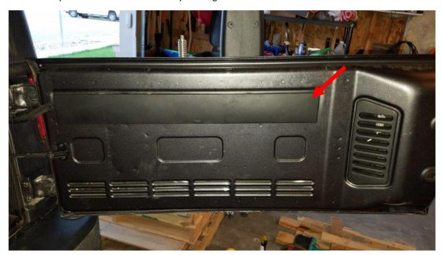
**10.** I recommend wrapping the colored wires in electrical tape for a cleaner finished look. Then hold up the table in the desired location. Make sure it will clear the floor and any soft top hardware when the tailgate is closed. Then mark your desired bolt locations. Then center punch the marked locations for drilling.
