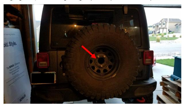
8. Using a 13mm socket remove the 8 bolts attaching holding your spare tire carrier to the tailgate and remove the spare tire carrier. Then remove the plastic vent grill behind it. This will give you a view inside your tailgate to make sure you don't drill in the wrong place. Note: After learning the hard way, I highly recommend this step.
