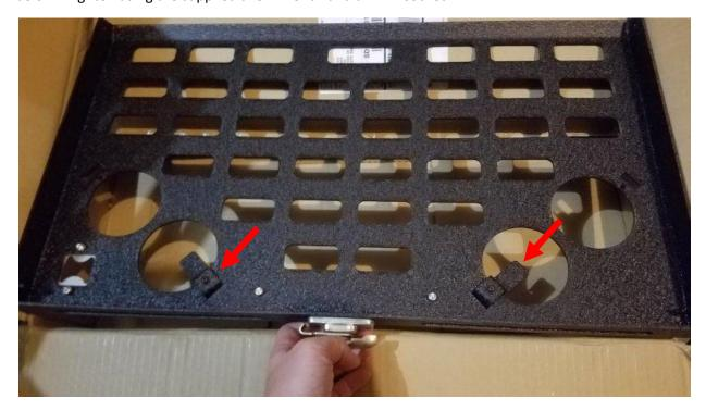
3. Next you will attach the swing arms to the base. Looking at the picture below I will list from top to bottom what hardware is installed. 6mm x 80mm bolt, washer, nylon flange sleeve washer (smaller portion facing upward), rubber sleeve, nylon flange sleeve washer (smaller portion facing down), washer, 6mm nylock nut. Build all 4 hinges in that order, and hand tighten the nut for now.
