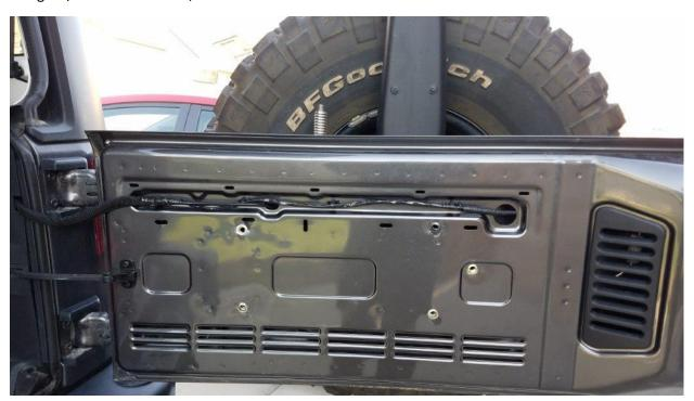
**15.** Lift the table into place and hand tighten the 4 supplied 3/8" x 1" bolts with washers. *Note: It helps to have a separate set of hands to hold the table in place.* Then use the supplied allen wrench to tighten all 4 bolts. Be careful not to overtighten or the nutserts could become loose and start to spin.
