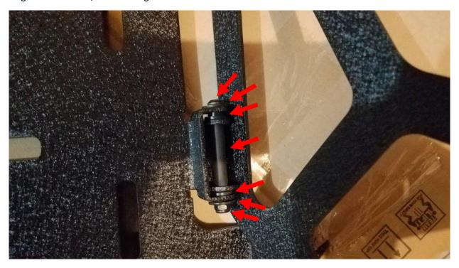
**4.** The swingarms should look like this. Now using the supplied allen wrench and a 10mm socket, tighten all 4 hinges until the swingarms move smooth with slight resistance.
