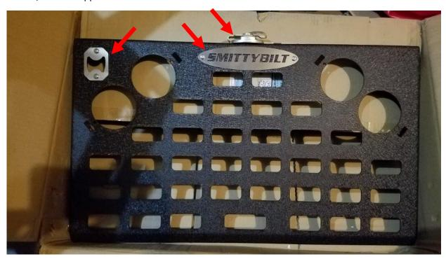
2. If you will be using the cup holder attachments, install them now. I chose to start with 2 and see how I like them. Using the supplied 10-24x1/4" hardware (the smallest supplied nuts/bolts) install the brackets as shown below. Tighten using the supplied allen wrench and a 7mm socket.
