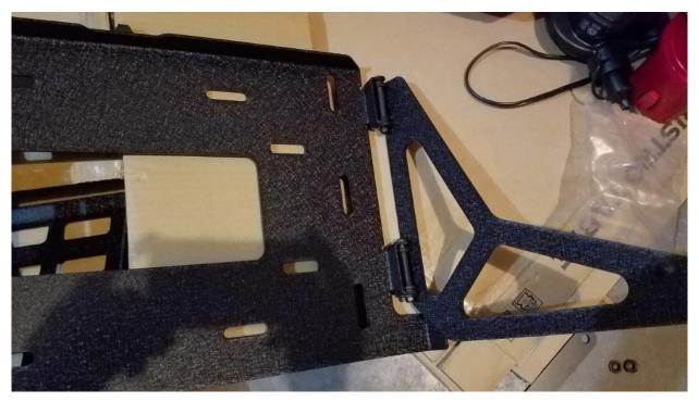
**5.** Next, install the supplied gasket to the back of the mounting base. This gasket sits between the mounting base and your tailgate. Wipe the base clean, peel the paper backing off the gasket, line it up as shown below, then press it down into place. .
