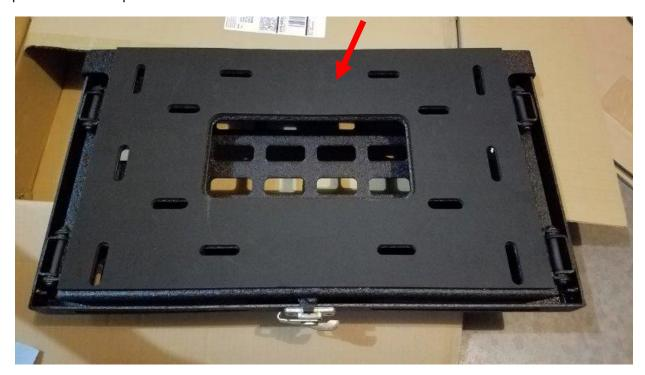
**6.** Now attach the table to the mounting plate. Use the supplied ¼"-20 x1" bolts and hardware. Install bolts on both sides of the table. Using the supplied allen wrench and a 10mm socket tighten until the table folds smoothly with slight drag.
