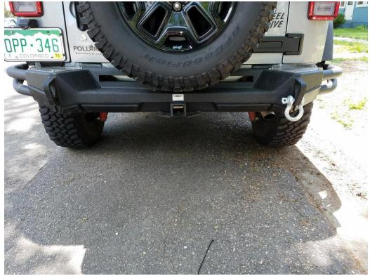
NOTE: The factory spare is pressing against the vertical part of the new bumper, with minimal pressure needed to close the tailgate. However, oversized width tires (ie greater that 255s will likely require modification to the spare mount to allow the tailgate to close properly.
