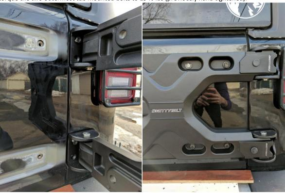
4. **Install the tire mount bracket** – Using the supplied 12mm bolts, washers, and nylon nuts, attach the tire mount bracket base to the tire mount bracket (18mm socket). If using the third brake light mount, attach this piece as well. Torque to 80 ft-lbs. Bolt these pieces to the tailgate and HD Tire Carrier using the supplied 8mm x 40mm bolts. Be sure to use the supplied spacers show below in the first picture. Torque to 15 ft-lbs.
