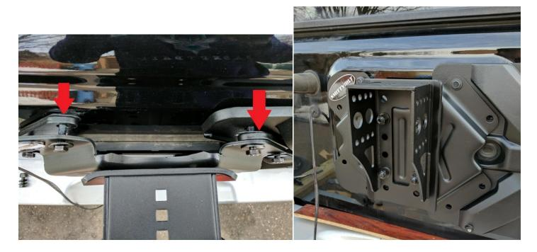
5. **Attach the tire mount** – Using the five supplied 10mm bolts, nuts, and washers, attach the tire mount to the tire mount bracket. Adjust as necessary to fit your wheel's offset/back spacing. Torque to 37 ft-lbs.
