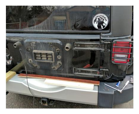
2. **Removing the hinges** – Before unbolting the hinges, support the tailgate by placing wood shims between the rear bumper and the bottom of the tailgate. This will prevent the tailgate from misaligning. Once in place, remove the tail gate hinges using a 13mm socket and T50 torx bit.
