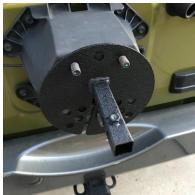
5. Install the tire back onto the carrier and re-install the wing nut.
