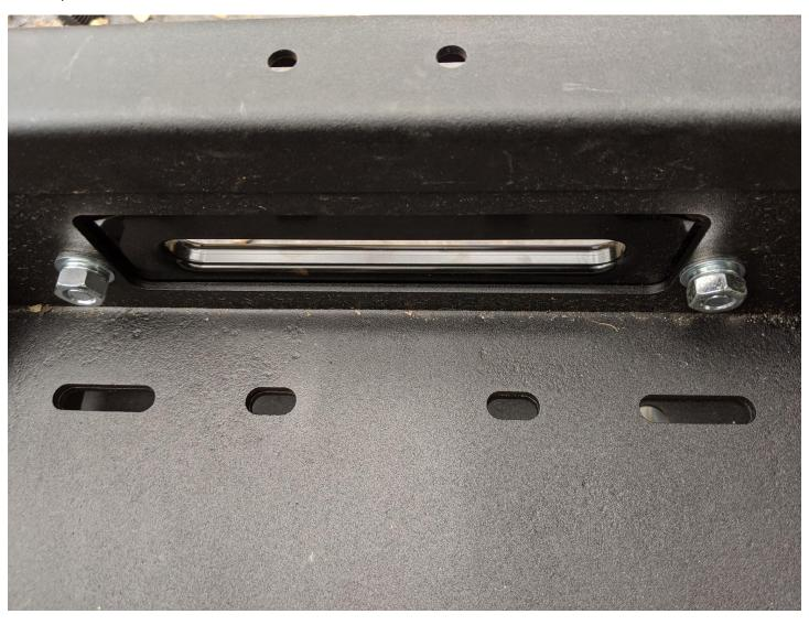
2. Determine whether you will mount the control box on top of the winch cage or on the side of the winch. It is typically easier to install the box prior to mounting the winch. The following instructions will dictate a cage mount configuration.
