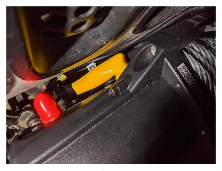
6. After centering winch cage with fairlead, install (4) flat washers, lock washers, and bolts from underneath.
