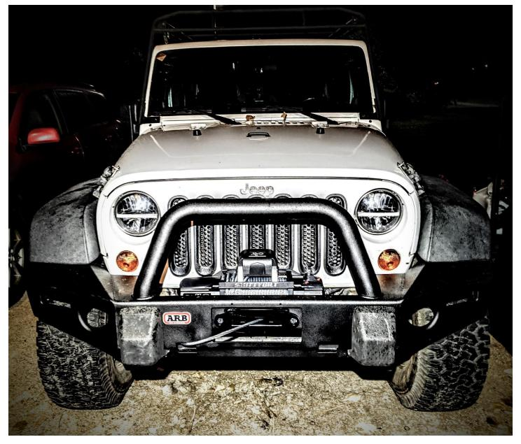
8. NOTE: As shown above, I opted to use a Hawse style fairlead in place of the provided roller fairlead. If going this route, ensure that the fairlead is rated for steel cable (usually cast iron vs alloy).
