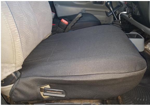
5. Slide seat back cover over the seat back. Make sure the tilt lever does not get hung up on the cover and the Velcro does not get stuck on the seat back.
