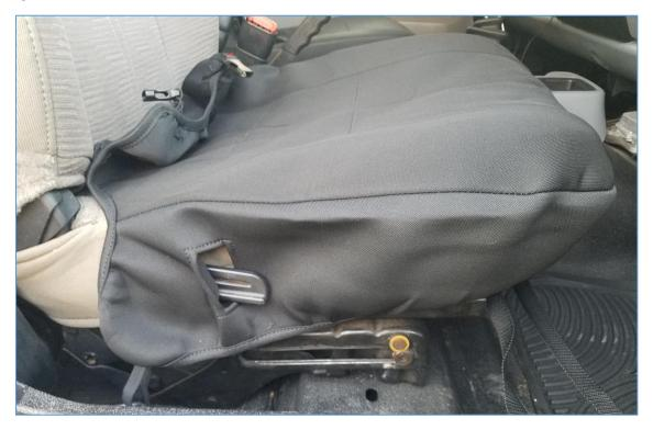
3. Tuck the buckle clasps under the seat back and feed the straps under the seat from the front to the back. Make sure not to tangle the straps in any of the moving seat parts or slide lever. Adjust cover positioning and connect the buckles.
