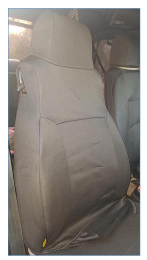
6. Adjust the fit and tuck the front flap under the seat back. Secure the Velcro to the front flap.
