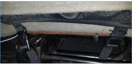
4. Tighten buckles and connect seat side cover retaining straps and hooks.
