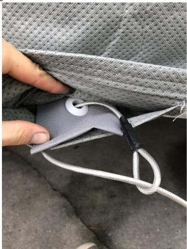
8. Finally secure the wire through the grommet on the driver side with the provided lock.
