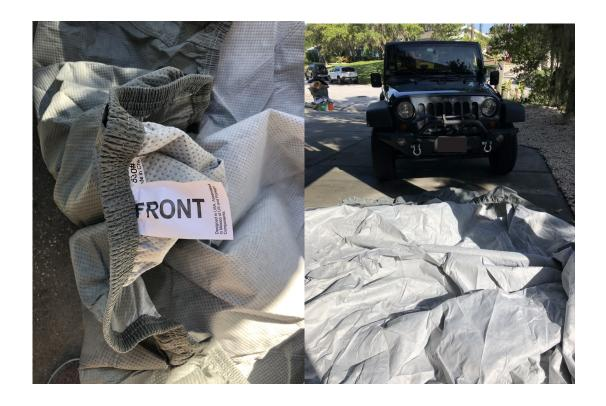
2. Take the rear end of the cover (the end you layed furthest away from your vehicle) and pull it over the car. If you have someone helping you then carefully continue to bring the end towards the rear of the car. If you are installing this alone you will have to constantly walk to the different side of the vehicle to evenly lay the cover over the car. (If You have lights or other accessories on you Jeep be careful that the cover doesn't get caught on them).
