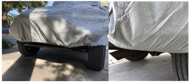
7. The cover comes with an included wire and lock to secure the cover to the vehicle. Insert the wire through the grommet on the passenger side.
