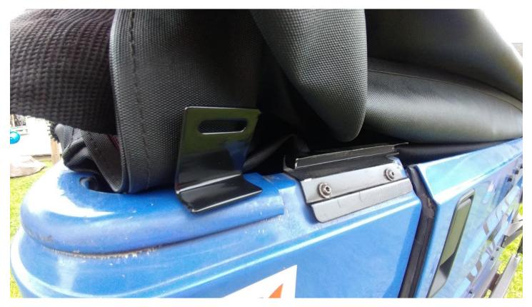
4. Loosely connect the rear straps to apply some tension to the front seam.
