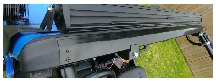
2. Start by putting the Smittybilt Extended Brief Top over the roll bars and pressing the front seam into the header. It will not stay.
