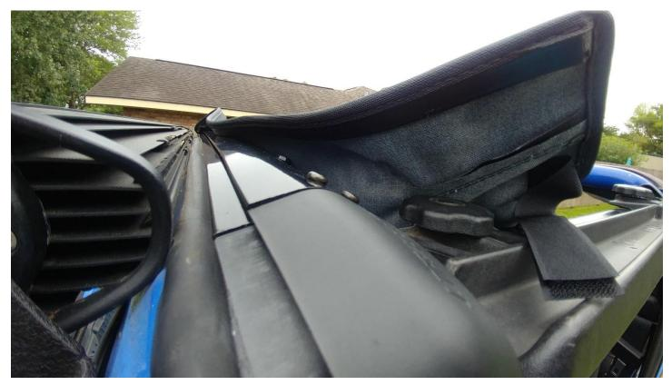
3. Locate and insert the angled clips for the rear straps.
