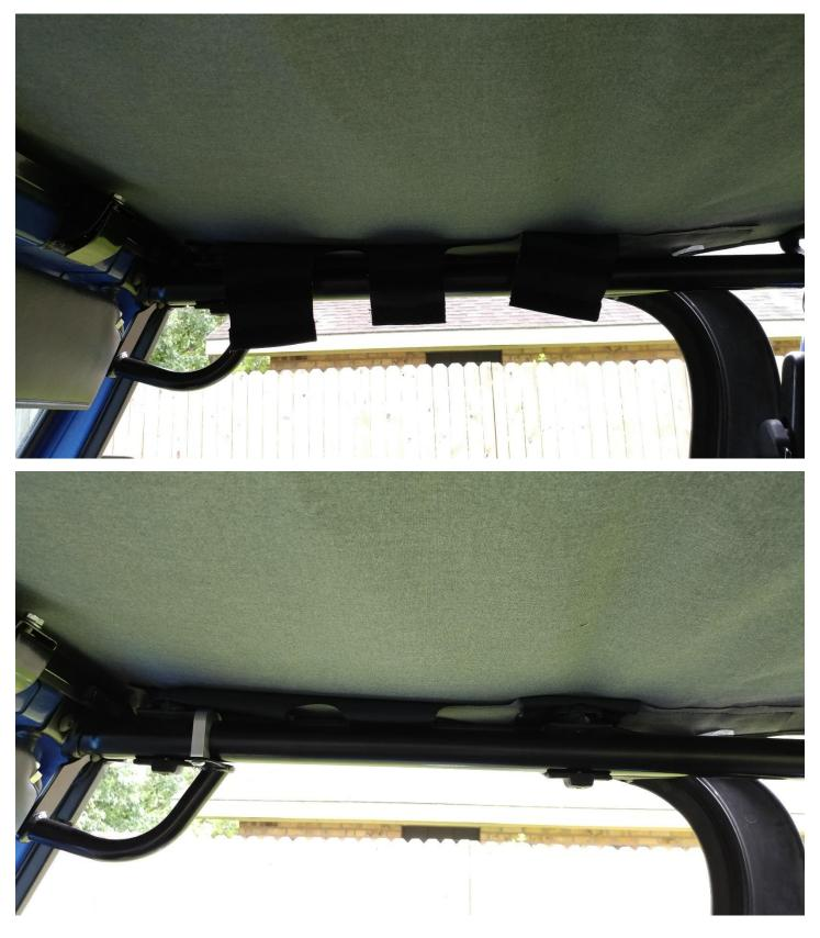
8. Secure the straps around the outside center roll bar
