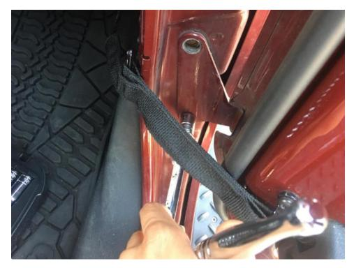
4. Remove the hinge and replace it with the corresponding bottom hinge. Tighten the interior 5mm screws, which have the rounded head, making sure to try and line up the new hinge with the outline of the old hinge.
