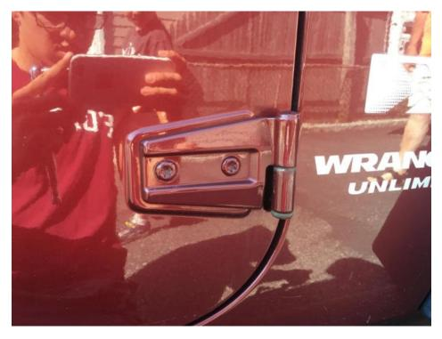
3. While having a second person hold the door, use the ½" socket to remove the two screws from the bottom hinge on the interior.
