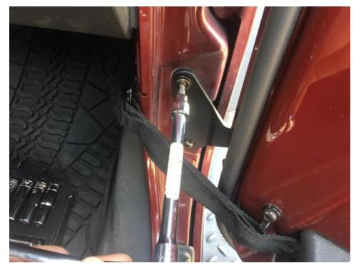
5. Tighten the 5mm flathead screws to the exterior of the door hinge.
