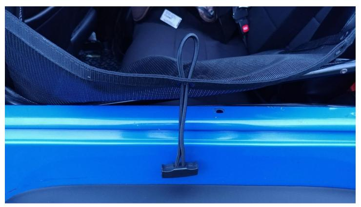
6. Hang the side mesh panel by wrapping the bungee around the roll bar
