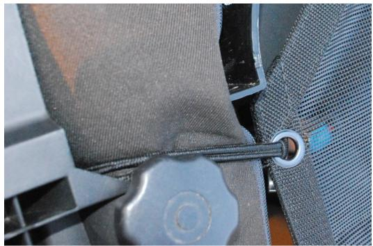
7. Note: To put the hard top or soft top back on, you will need to unhook the two front left and right rivets in order to fasten the top to the brackets. You can loop the elastic fasteners to themselves while the
