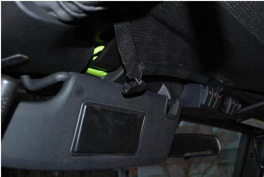
8. Make sure that none of the fasteners interfere with any safety equipment such as seatbelts, visors, mirrors, airbags, or any moving parts.
