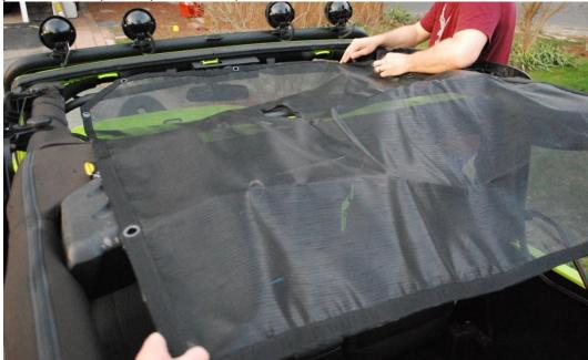
4. Fasten the three rivets to the three brackets above the windshield using the three short elastic loops – the needle-nose pliers can be used to feed the elastic loops through the brackets, if needed. Make sure the plastic handle of each elastic loop is underneath the mesh top, to avoid interference with your roof when it is being used.
