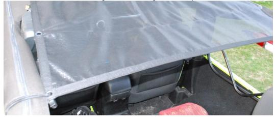
6. Working your way from rear to front, fasten each side until all the rivets have been secured with all of the elastic loops. Note: when you get to the front, make sure the loops are fastened around the roll bar, and *not* the frame for the door or any other equipment.
