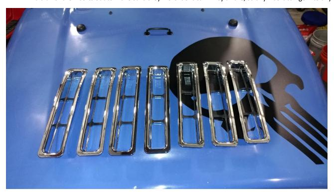
3. Notice the curve in the inserts. This must line up with the upper portion of the grill
