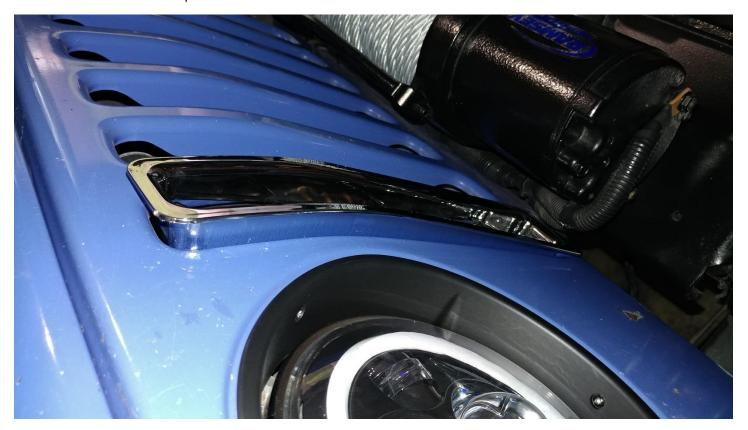
5. If the insert is not snapping in, remove it and start for the lower portion first. Do not apply to much pressure, they are plastic and the tabs could snap off.
