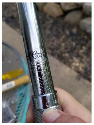
7. Tighten all four bolts, being careful to use either the clicking of your torque or the scale as a guide to avoid overtightening.
