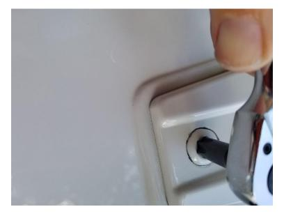
3. Place the gasket beneath the top edge of the step and hand tighten the T30 bolt that comes with the kit. There should be enough room to access the upper right T50 bolt for removal.
