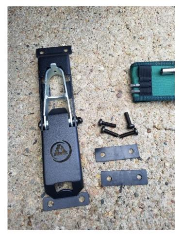
2. After scoring/breaking the paint as described in the pre-installation notes, remove the upper left T50 bolt.
