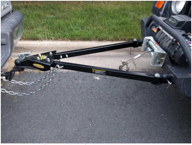
5. PRO TIP: For ease of lining up vehicles, use safety chain attached to Towed vehicle bumper to raise Tow Bar up and then move Towed Vehicle into position versus backing Tow Vehicle up to it. This allows you to see exactly where your hitch point lines up, making the process much simpler.
