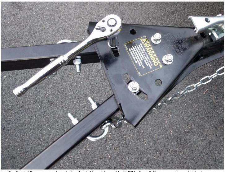
7. Smittybilt recommends replacing Quick Pins with provided 1/2" bolts at D Ring connection point for longer distance towing.
