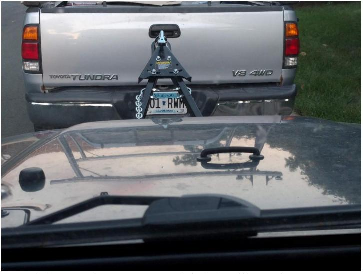
6. With all components of Tow Bar now in position, go back and Tighten all fasteners with appropriate socket/wrench. Adjust hitch to ball connection as necessary to ensure a secure connection.
