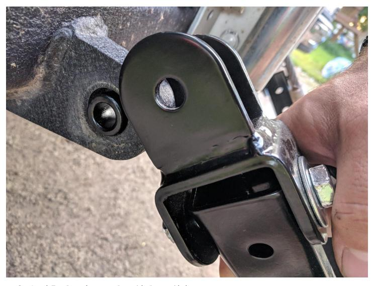
3. Attach Tow Bar to bumper using quick pins provided.
