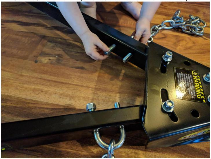
2. After removing recovery shackles (if installed), insert spacer sleeves into mounting points on bumper.
