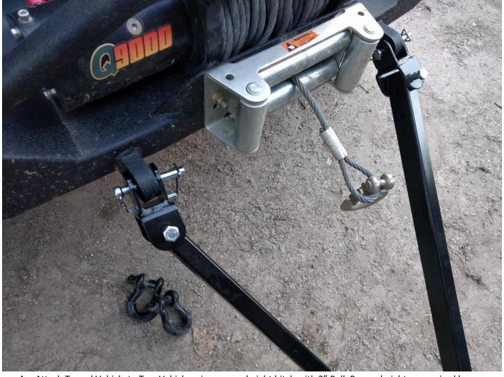
4. Attach Towed Vehicle to Tow Vehicle using proper height hitch with 2" Ball. Proper height as required by Smittybilt is maintaining no more than 10 degrees from level across the Tow Bar between vehicles. Attach safety chains to Tow Vehicle and insert Quick Pin into Tow Bar Hitch to Secure.
