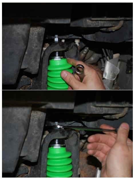
15. Extend the shock by hand and line up the bottom of the shock with the lower shock mount.16. Reinstall the original lower shock mount bolt and tighten with an 18mm Socket and Torque to 90 lb/ft.
