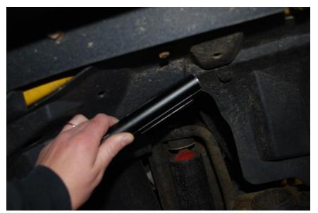
12. Remove the shock making sure you remove both of the rubber grommets from the upper shock mount.
