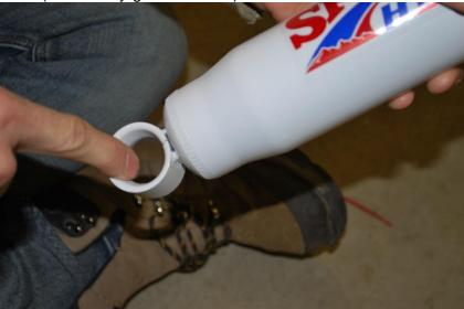
4. Apply a liberal amount of dish soap in the bushing and press the inner bushing into the rubber bushing with your hand.
