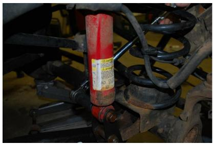
12. Using 2 16mm Open End Wrenches (or a 16mm and a 5/8), remove the upper shock mounting nut. This can be tedious. In the pictures, vice grips were used, this can also substitute one of the wrenches.
