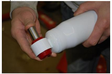
6. Install the shock boot and secure with the provided zip tie. Trim the excess zip tie with wire cutters.
