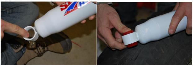
5. Apply a liberal amount of dish soap in the bushing and press the inner bushing into the rubber bushing with your hand.
