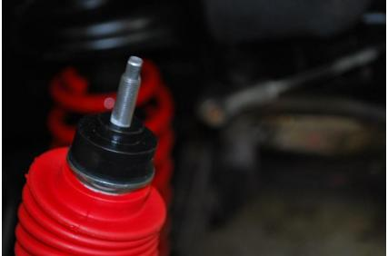
15. Place the other grommet on the upper shock bolt and tighten the upper shock nut until the upper mounts expand to about the same diameter as the washers using a 7/16 Open End Wrench.
