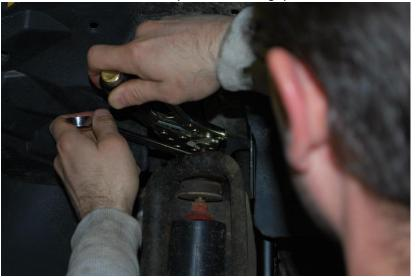
13. Remove the shock making sure you remove both of the rubber grommets from the upper shock mount.
