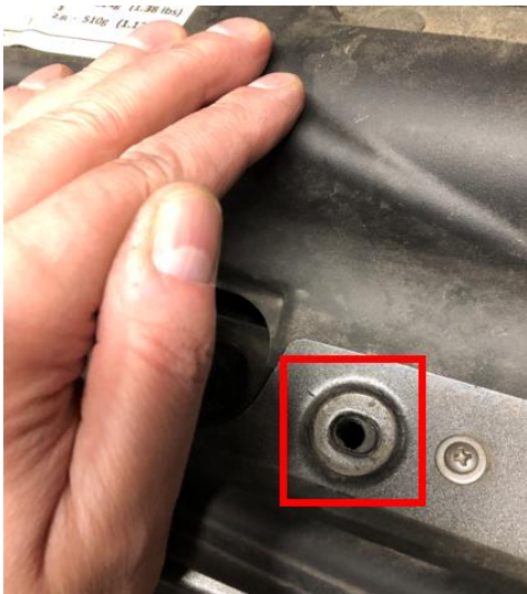
Align holes in top of grill for clip placement
