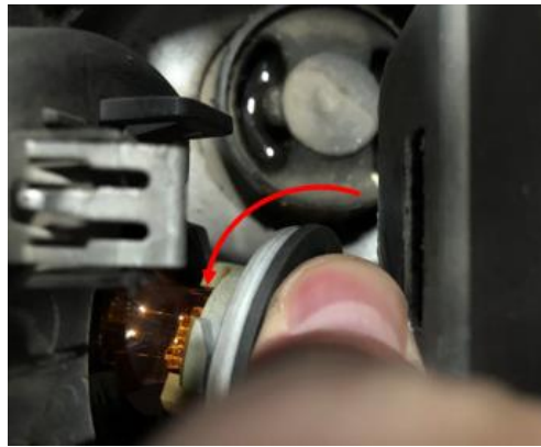
Twist 90 degrees and pull to release from grill
