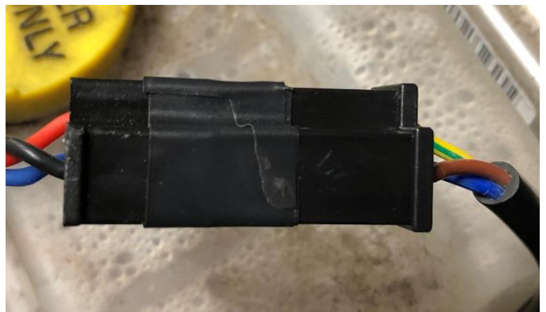
Use electrical tape to seal the connection
