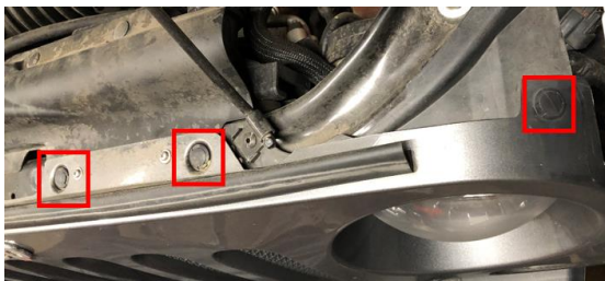
Find the tabs holding the grill in place
