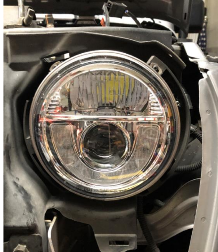
Mounted headlight with all screws tightened
