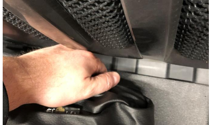
Push gently on bottom of grill to seat clips
