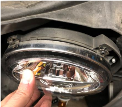
Insert headlight and tighten screws halfway
