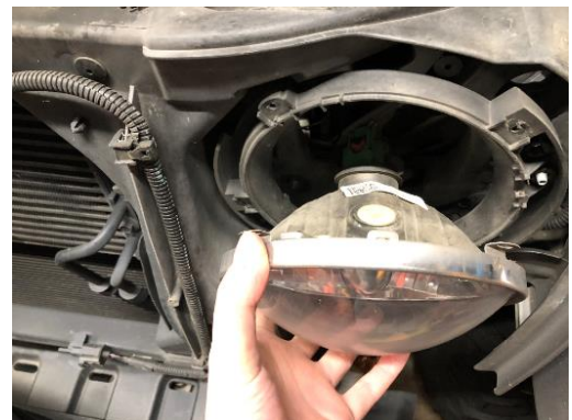
Pull headlight out slightly
