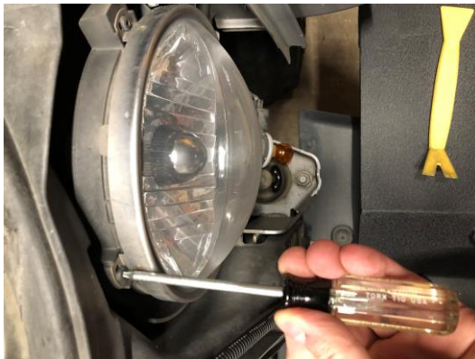
Remove 4 screws with Torx T10 driver
