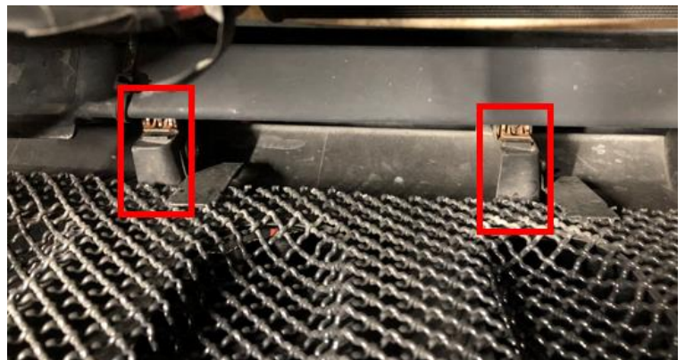
Metal clips in radiator frame
