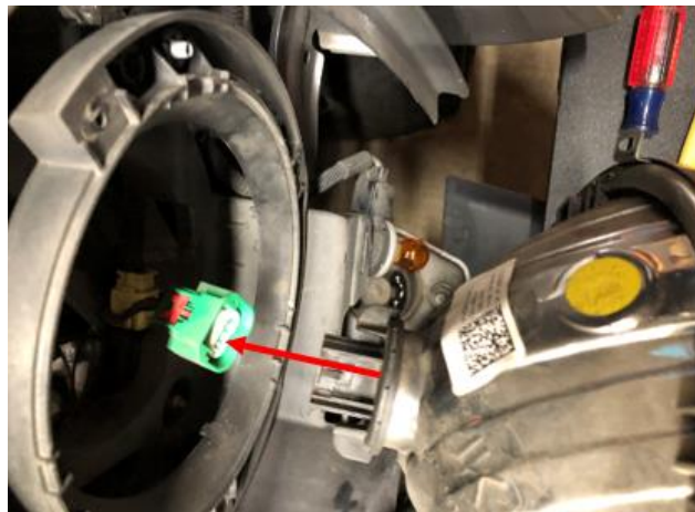
Pull plug away from headlight
