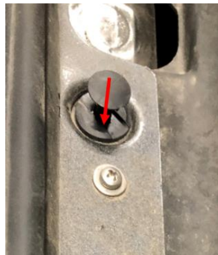
Insert clip and press on center until it seats
