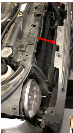
Grill pulled away from the radiator frame
