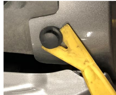
Use pry tool to remove the tabs
