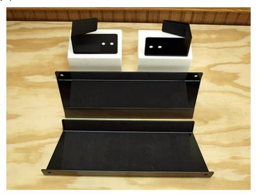
Note: You will need to purchase eight (8) 5/16" lag bolts at least 2-1/2" long and eight (8) 5/16" flat washers from your local hardware store. Lag bolts and washers are NOT supplied with the brackets. The lag bolts that were used for this install had a 1/2" head and were 2-1/2" long. Also, the holes in the Lower Brackets are made for 16" on center studs. You will need to determine additional materials to appropriately secure the brackets if your wall has 24" on center studs.
