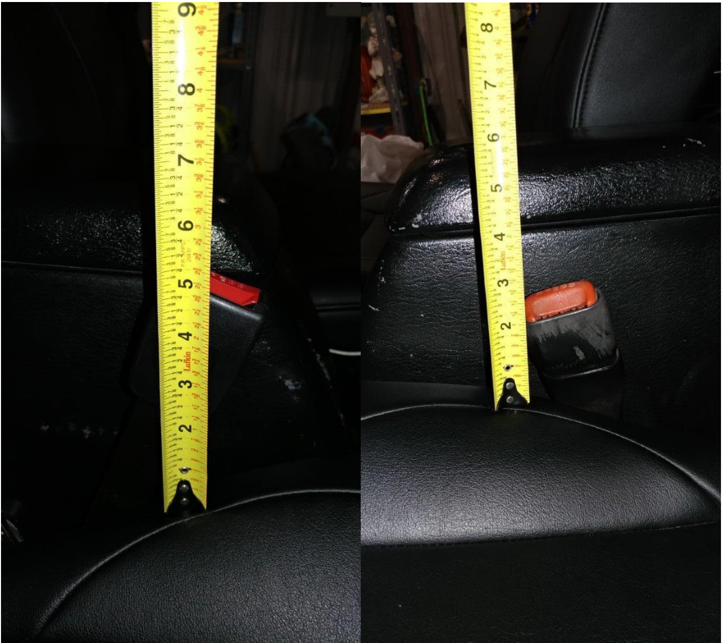
16. The new lower seat belt latch receiver height compared to factory.
