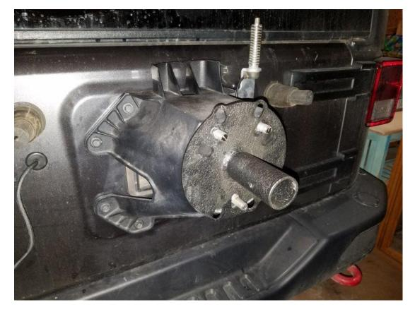
**3.** Put the spare tire back in place with the bracket through the center of your spare wheel. Use a 19mm socket to tighten the lug nuts holding on the spare tire.
