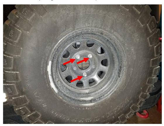
**2.** Place the base of your new bracket on the spare tire mounting bolts as shown.
