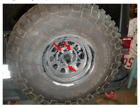
**4.** Next, install the removable part of your new bracket in the desired position. I chose to install it upside down to center the license plate in the spare tire. Insert the quick removal pin and secure it as shown.
