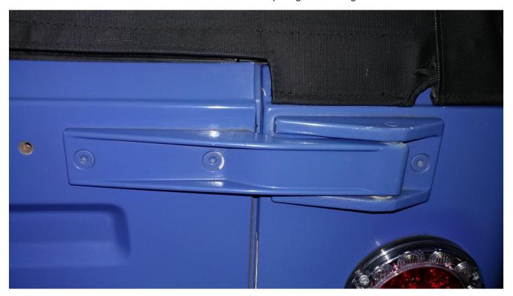
3. The surface underneath the hinge may need to be cleaned.
