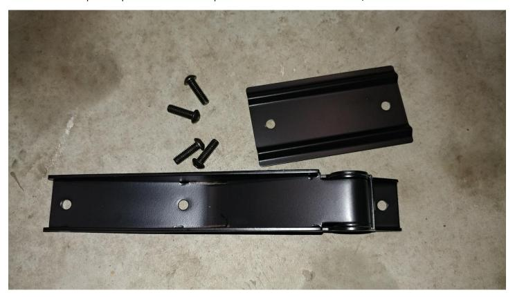
5. The backing nut/plate will move when the screws are removed. I found that even after trying to remove only one hinge at a time, I still needed to leave the 4 screws on the tailgate loose so that I could use a large flat head screw driver to level the tailgate.
