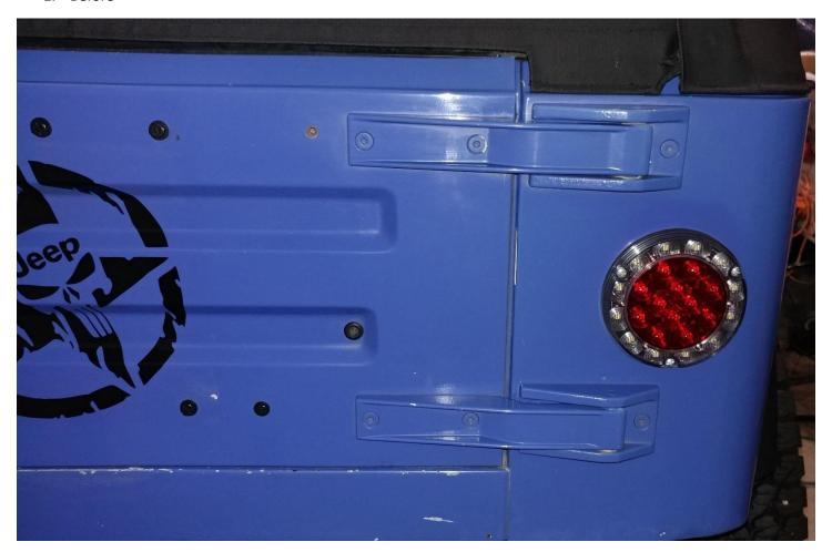
2. Remove the 4 T40 star bit screws. One is located after opening the rear tailgate
