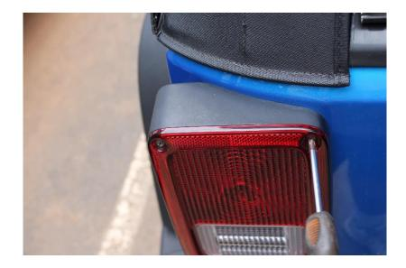
3. Note that inside screws are a different size than outside. Inside screws are smaller but longer.
