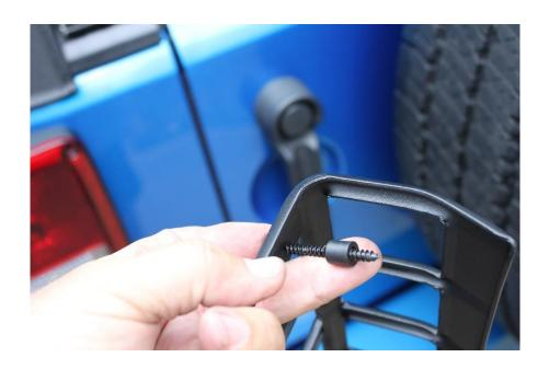
6. Position the guard on the lens and start the screw but do not tighten at this time.
