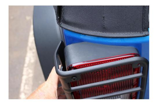
7. With the spacers between the lens and the guard start all the screws. Do not tighten until all screws are in place.
