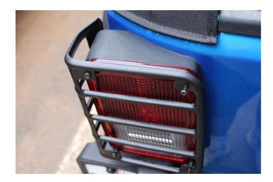
8. Working around tighten all the screws. DO NOT OVERTIGHTEN. You may be tempted to use an electric screw driver or a drill. If you do make sure the final tightening is by hand. Otherwise you may crack the lens.
